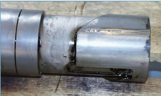
Fig. 2: Damaged plunger of injection pump
