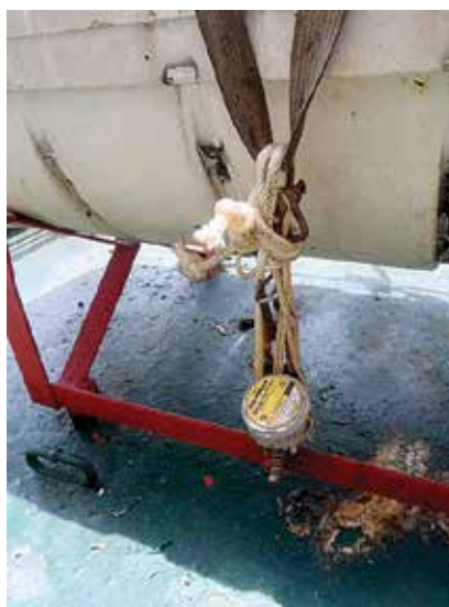
Defective Hydrostatic release
