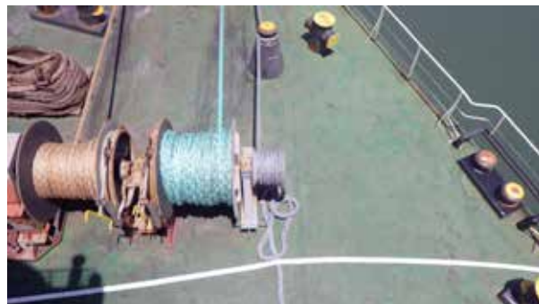
Mooring lines secured on warping drums
