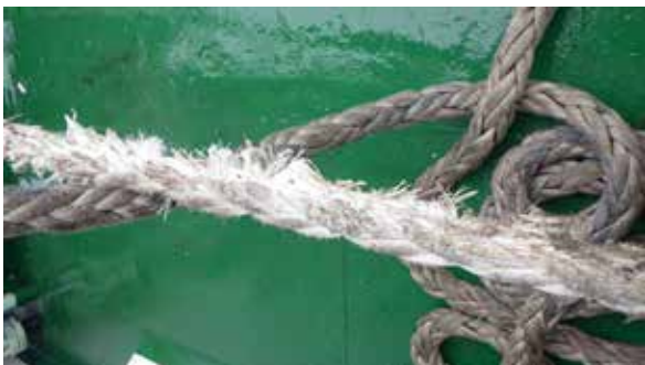
Damaged mooring lines
