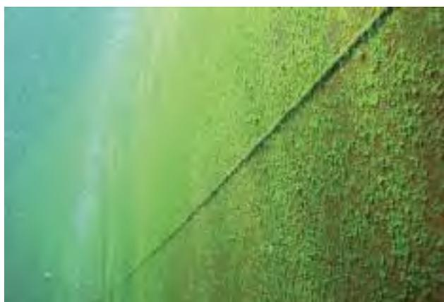
In addition, as the coating is soft, cleaning has to be effected by soft brushes or other non-contact methods, which can take more time and is more expensive than with other more conventional cleaning techniques.
