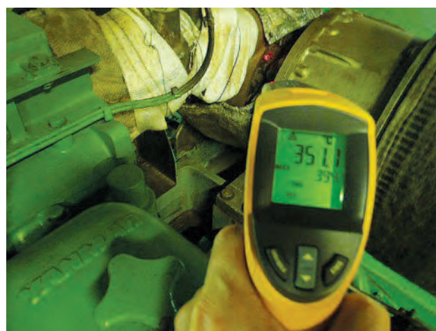
"Hot spot" due to missing insulation
