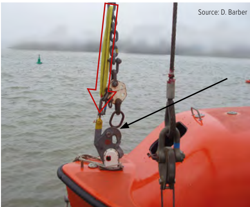
Alternative load path (arrowed Red) provided by a sling type FPD where disconnection of the main load path (hook and link arrowed black) has taken place.
