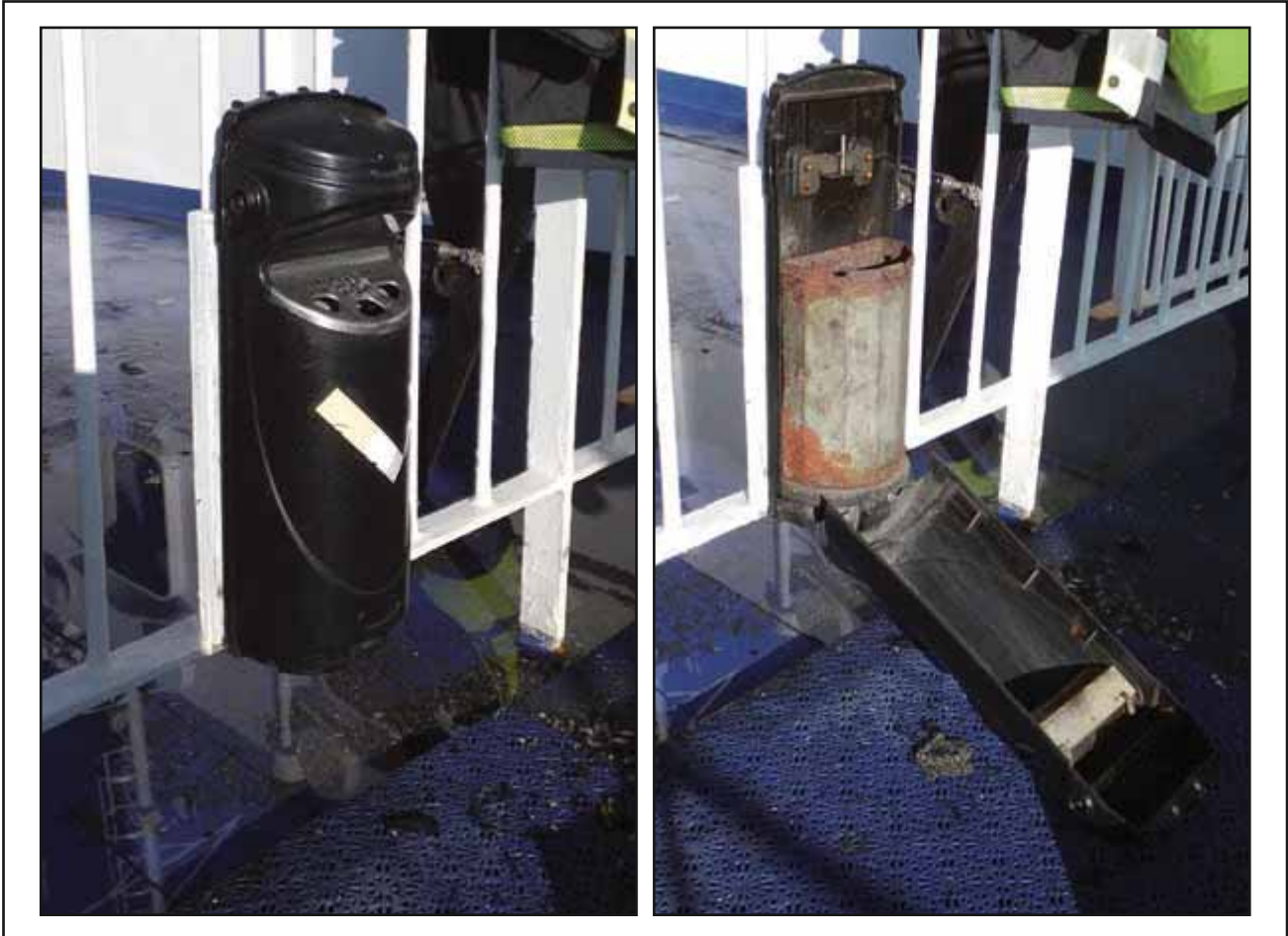
Figure 2: Cigarette bin and open bin with liner, which was missing from the bin that caught fire
