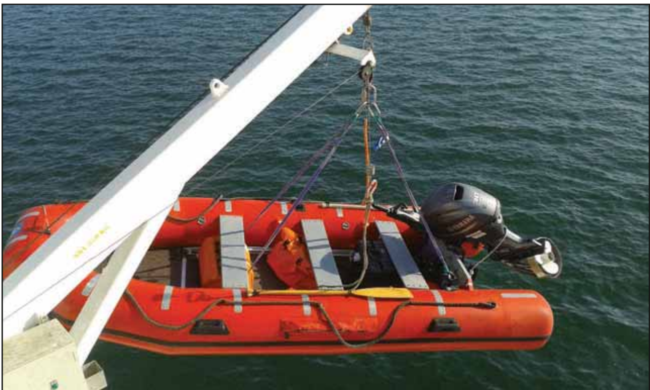
Figure 2: Lifting straps correctly fitted to inflatable rescue boat
