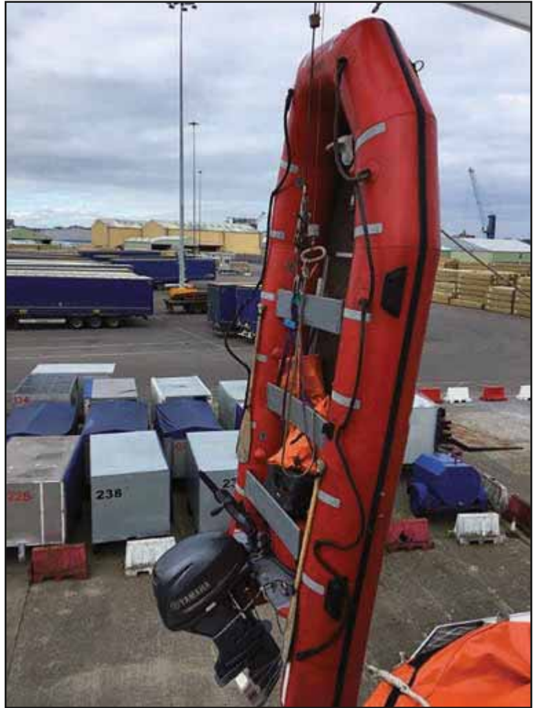
Figure 1: Lifting straps incorrectly fitted unbalance the boat and cause it to flip up
