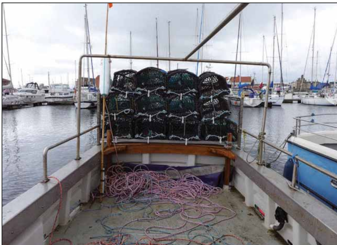
Figure 1: Reconstruction of the deck at the time of the accident showing the hazard associated with loose ropes
