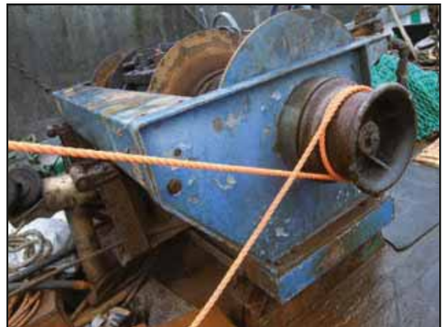
Starboard whipping drum with 1.5 turns of rope
