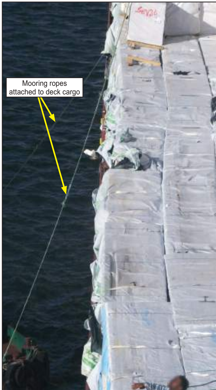
Figure 3: Cargo barges secured to deck cargo packages
