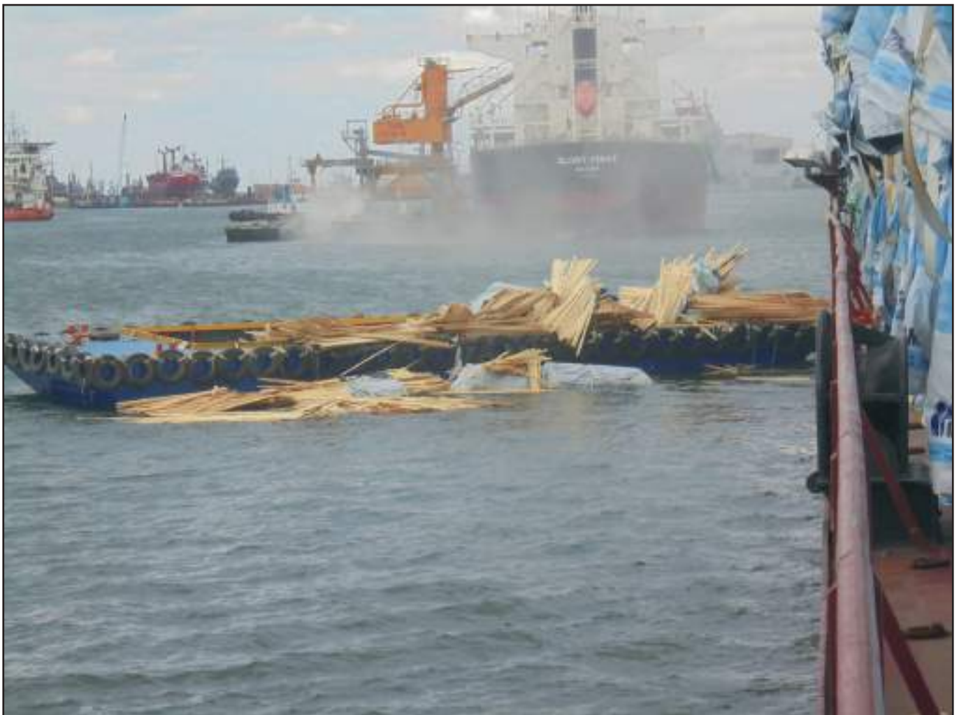
Figure 4: Port side cargo barge, immediately after cargo collapse
