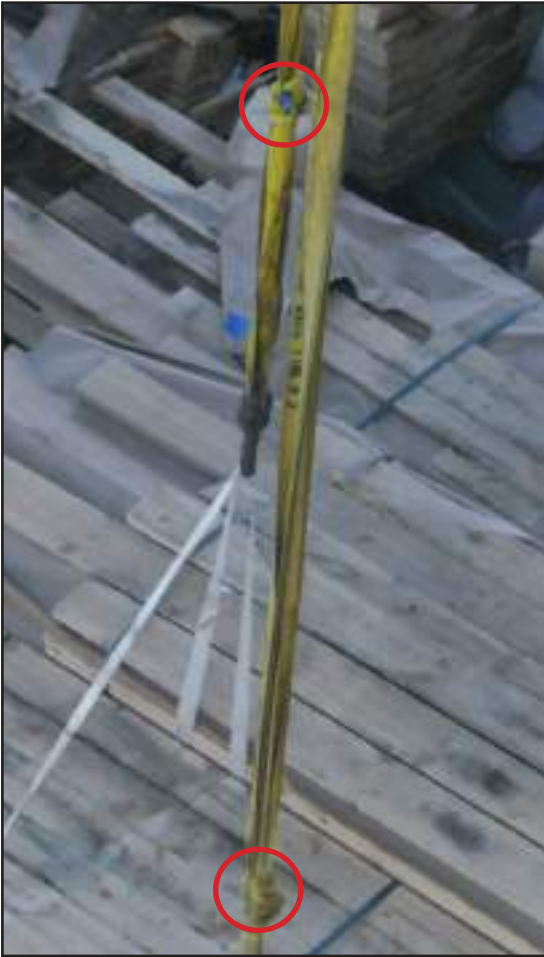
Figure 5: Knotted cargo slings
