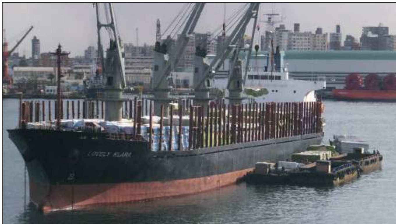
Figure 10: A vessel, with steel uprights, discharging a timber deck cargo at the same anchorage
