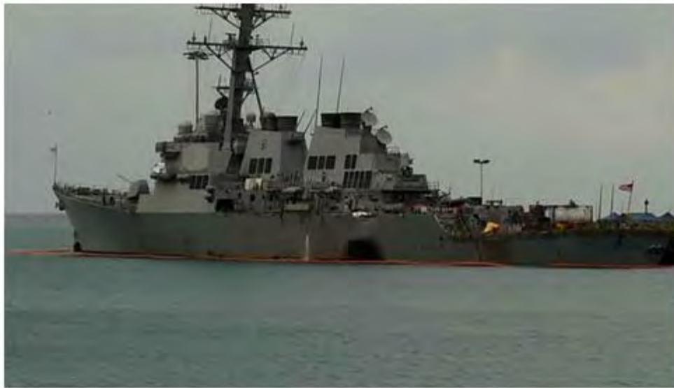
Figure 19 – Port side of JOHN S MCCAIN post-collision
