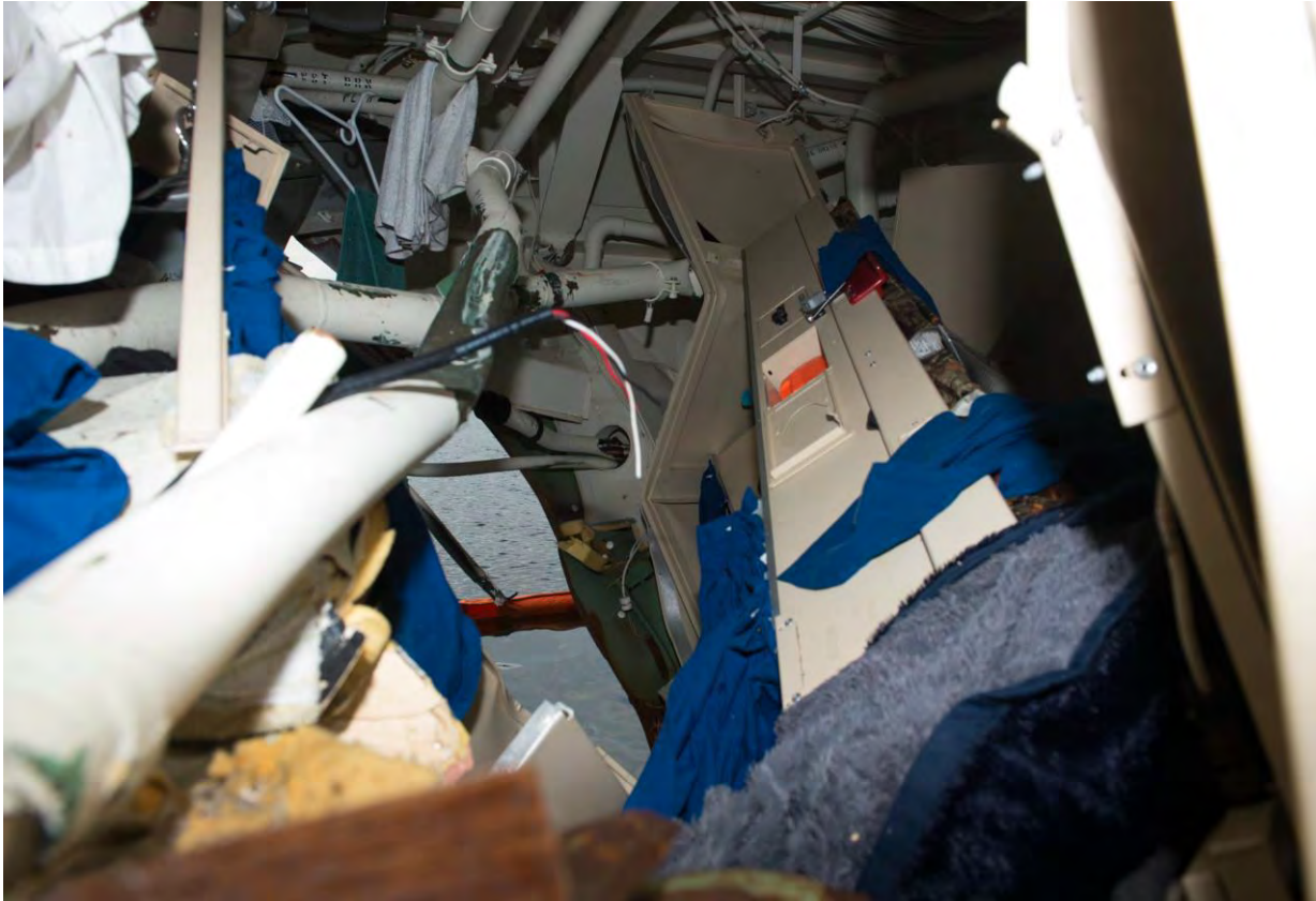
Internal view through Berthing 3 to point of impact; ocean visible
