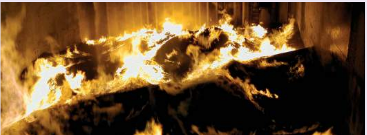
DRI which has self heated (Image courtesy of Burgoynes)
