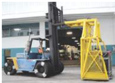
Forkliftcages used to transfer baggage around cruise ship terminals.
