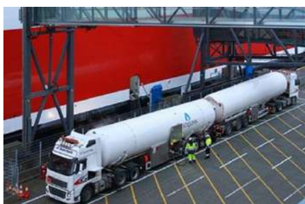
Figure 2.29 and 2.30 – LNG trucks in bunkering operation – From the top, LNG truck bunkering with second truck-trailer for Nitrogen/Inert Gas supply. Below 2 (two) LNG trucks bunkering back-to-back via common 2-way manifold derivation.
