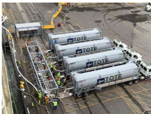
Figure 12.5 and 12.6 – TTS Bunkering by multiple trucks, via common manifold. It can be seen how the complexity of the operation is increased, not only with significant number of connection to common manifold but also with a significant number of personnel. To the technical challenge there is also an organizational one.
