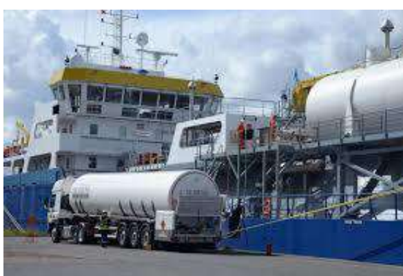
Figure 12.1 – TTS Bunkering. Truck-to-ship LNG delivery of LNG, with truck ashore, alongside of the ship, at berth.
