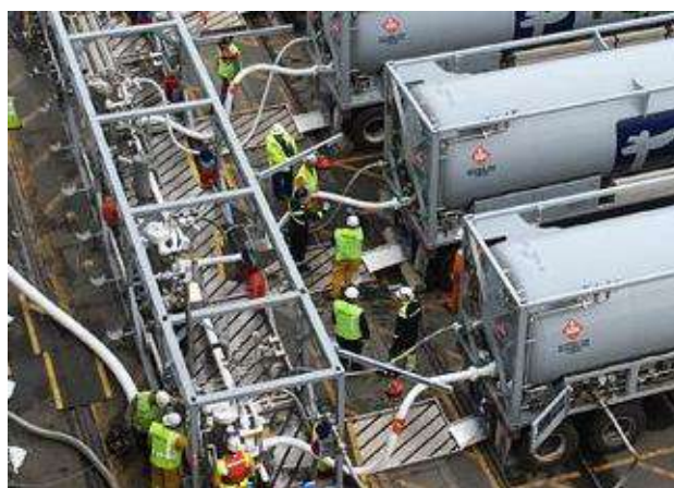
Figure 12.5 and 12.6 – TTS Bunkering by multiple trucks, via common manifold. It can be seen how the complexity of the operation is increased, not only with significant number of connection to common manifold but also with a significant number of personnel. To the technical challenge there is also an organizational one.
