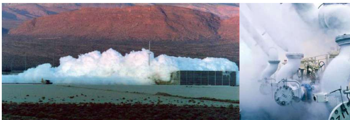
Figures 2.13 and 2.14 – LNG cloud formation and progression (on the left) opposed to the condensation cloud formation around LNG piping due to water vapour condensation in the air surrounding the cryogenic cold piping system.
