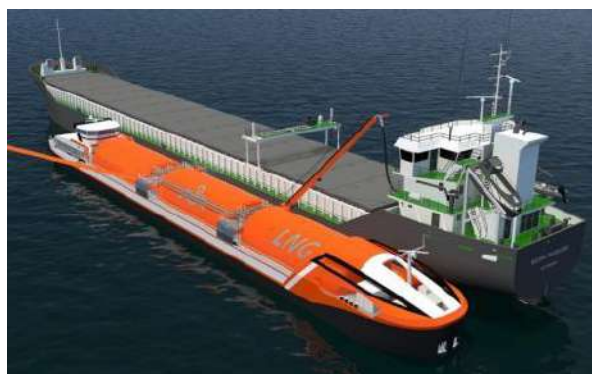
Figure 4.15 - Ship-to-ship LNG bunkering – riverine LNG bunker vessel to receiving ship
