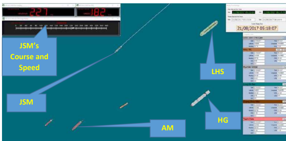
Figure 6 - Graphical representation of position of AM in relation to JSM at about 0518H
