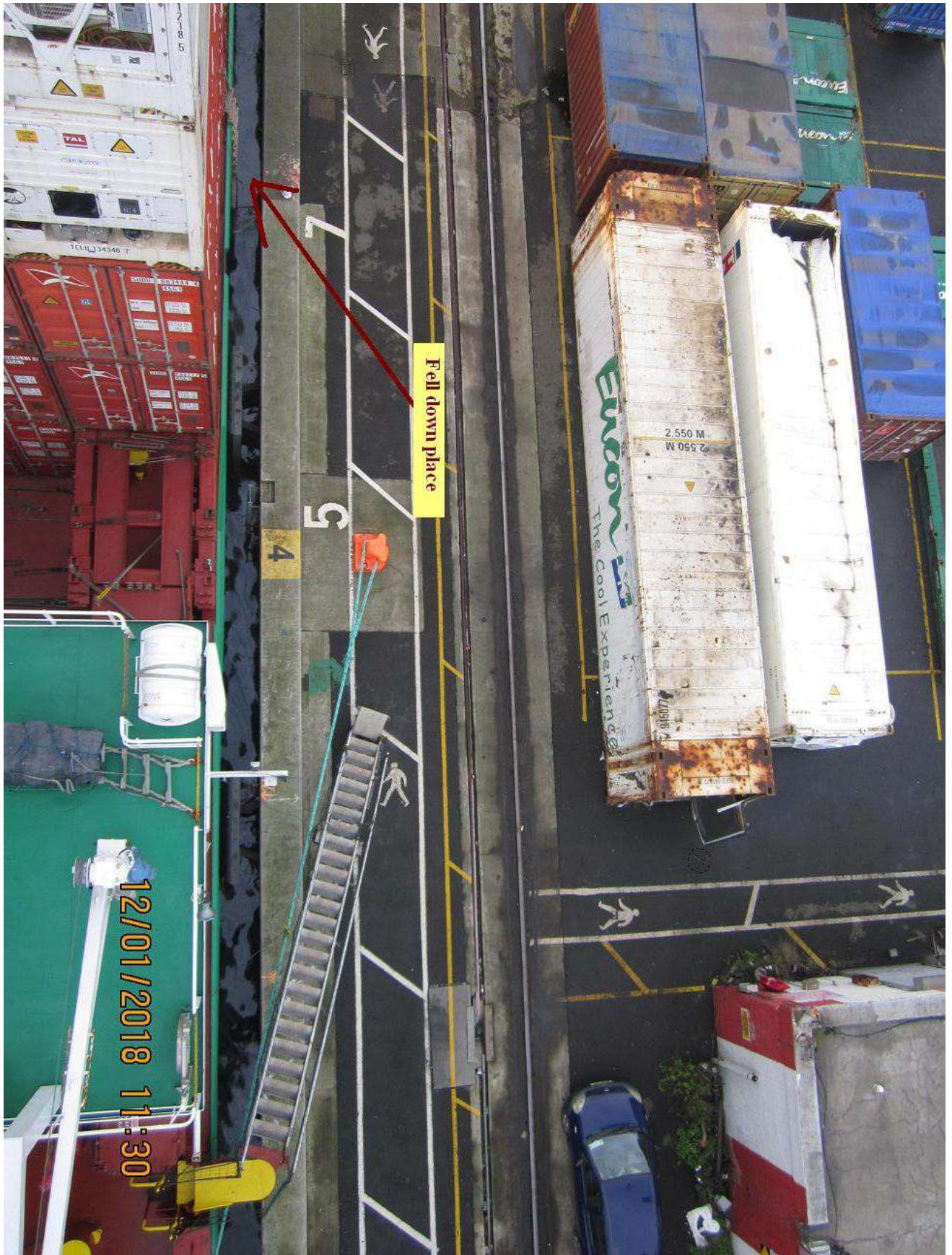
Fall down place indicated by arrow. A rope attached on the gangway's lower platform can be pulled for gangway's positioning on the quay.
