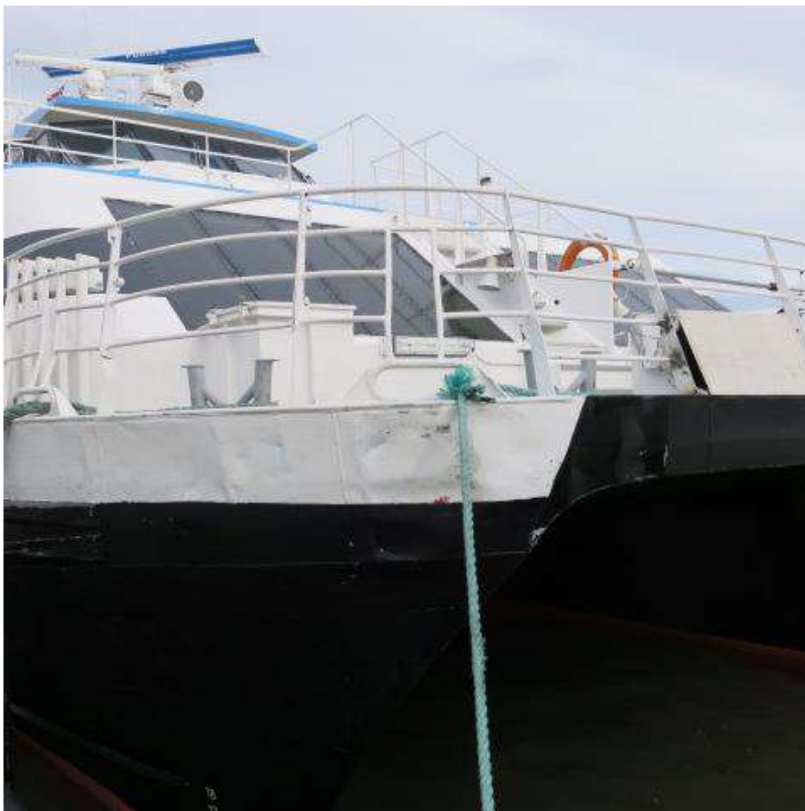
Figure 4: Aurora Explorer at the quay in Longyearbyen after the collision. The collision with the quay in Barentsburg caused only minor damage to the starboard hull and searchlight. Photo: AIBN
