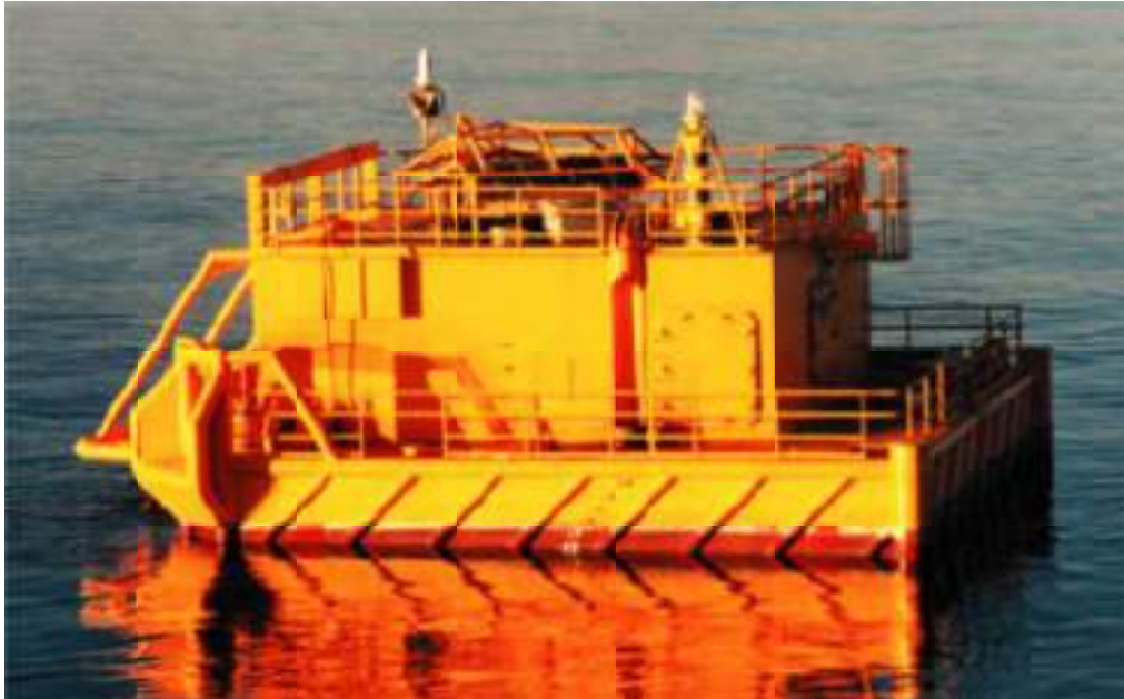
Figure 7 A Catenary Anchor Leg Mooring buoy
