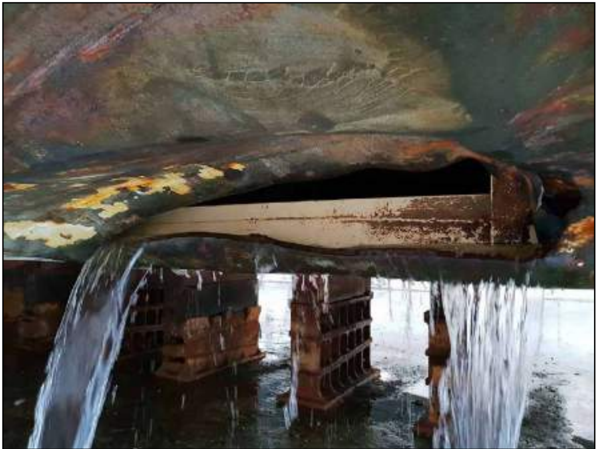
Figure 6: Priscilla - detail of hull damage
