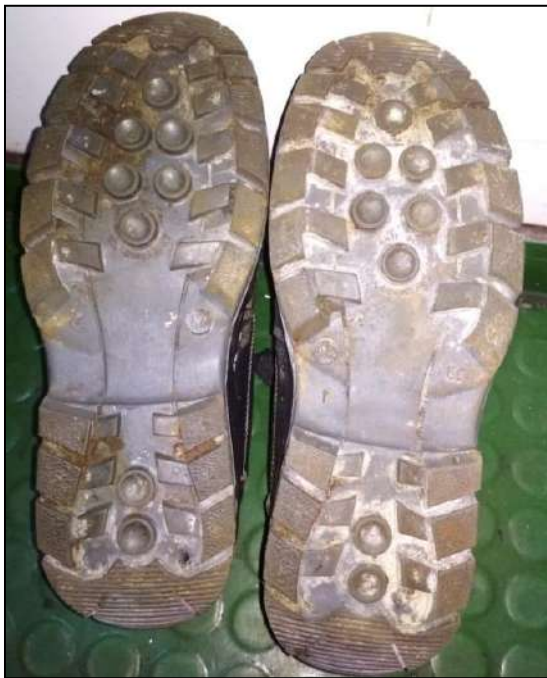
Figure 7: Grooves in the sole of the second engineer's safety boots
