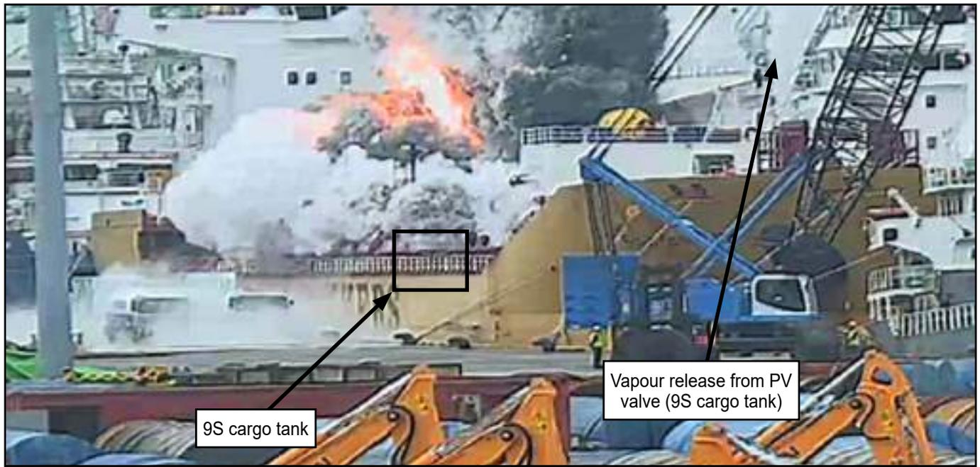
**Figure 1:** Tank rupture and ignition of released vapour
