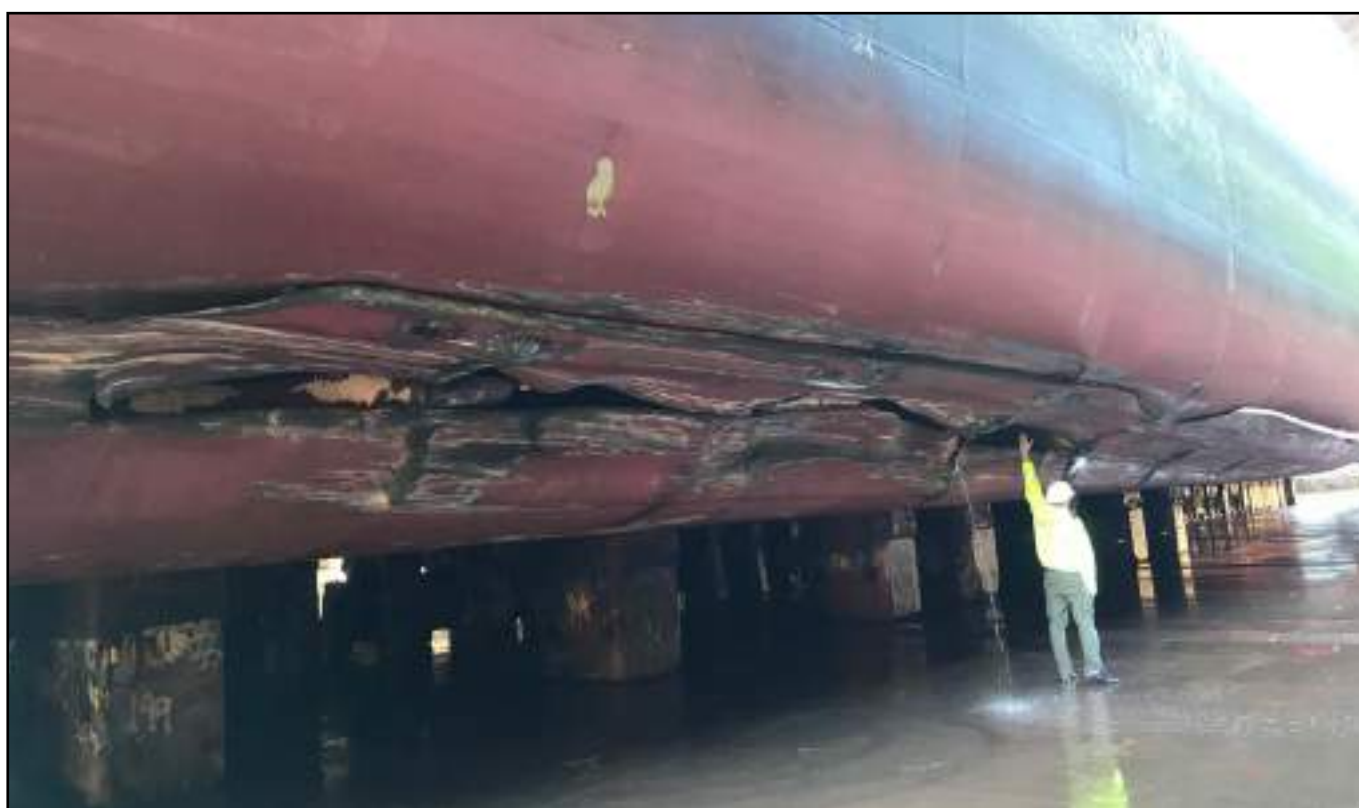
Figure 4: Damage to Seatruck Performance port side
