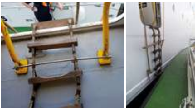
Completely illegal and highly dangerous method of rigging a pilot ladder
