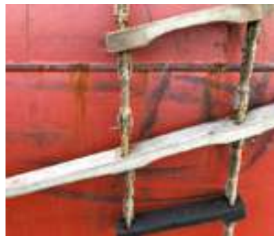
Figure 10 – Pilot ladder steps not horizontal, chocks missing. Ladder needs replacing
