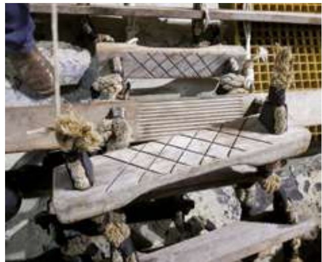
Deathtrap – pilot placed his weight on this ladder prior to disembarking and both side ropes parted!!
