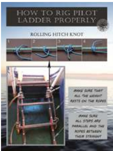
Figure 4 – A simple illustration of how to correctly rig a pilot ladder at deck level
