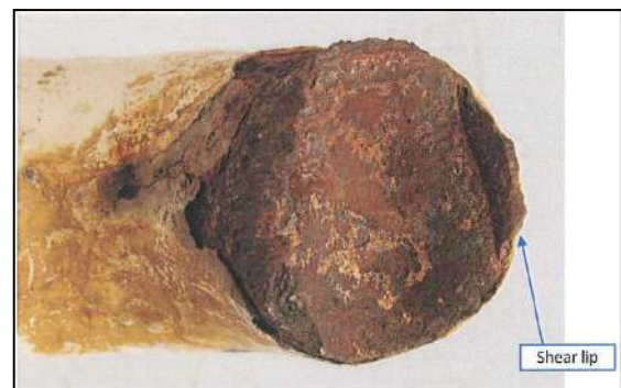
Figure 9: Macrophoto of fracture side B, magnification approximately 3.3X
