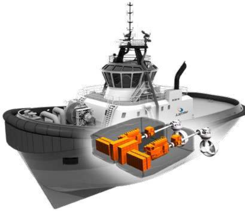
Figure 5: Wärtsilä HY system installed in a harbor tug vessel.
