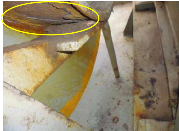
Poorly maintained windlass brake.
