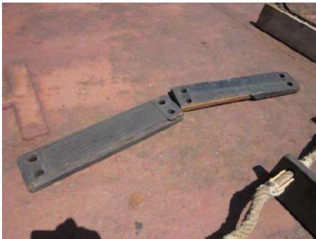
Broken pilot ladder.
