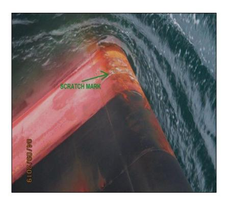
Figure 6: Superficial scratch marks on *Kanala*'s stem and starboard side hull *Source: Executive Shipmanagement Pte Ltd.*
