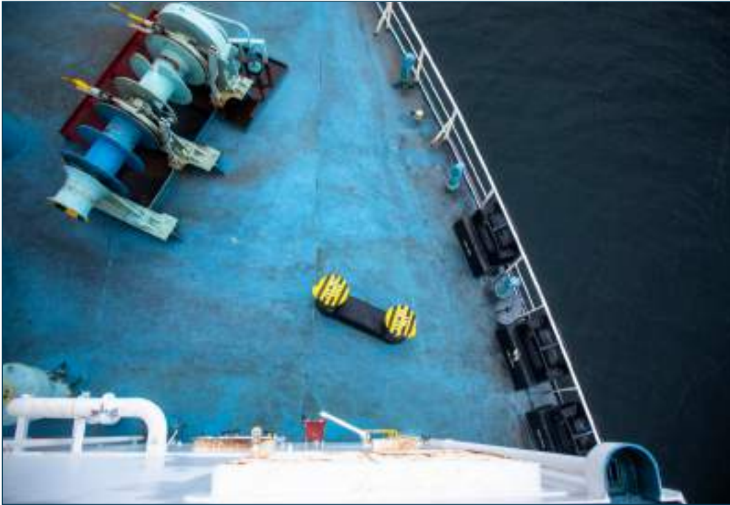
Figure 14: Mooring arrangement aft deck port side Source: DMAIB
