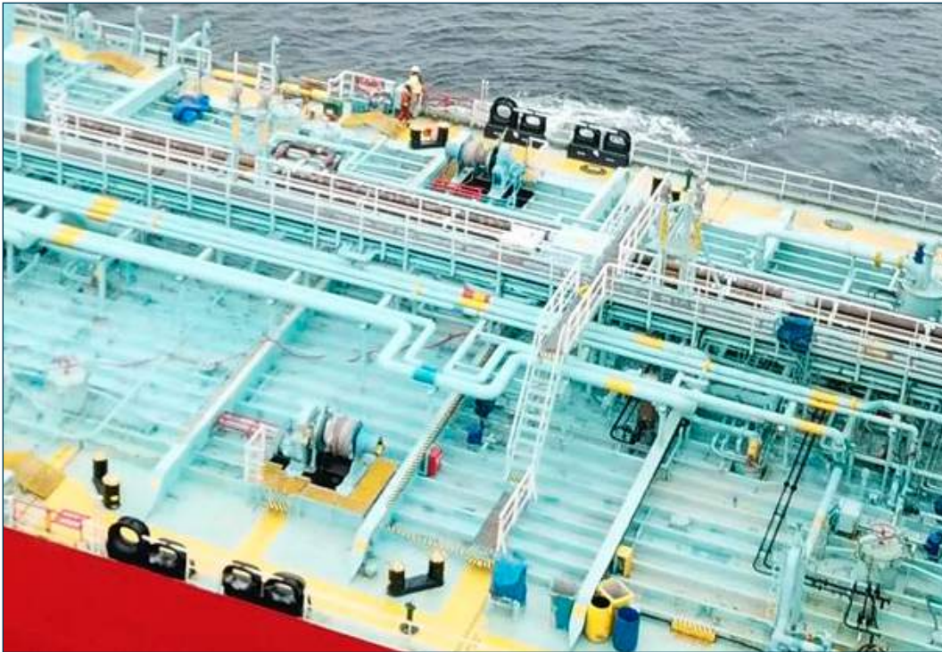
Figure 15: Mooring arrangement on the main deck Source: DMAIB
