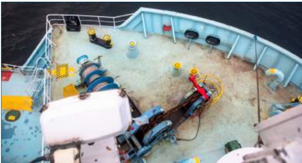
Figure 16: Mooring arrangement forecastle port side Source: DMAIB
