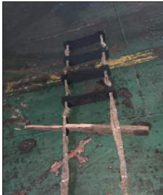
Figure 8: Damaged port side pilot ladder
