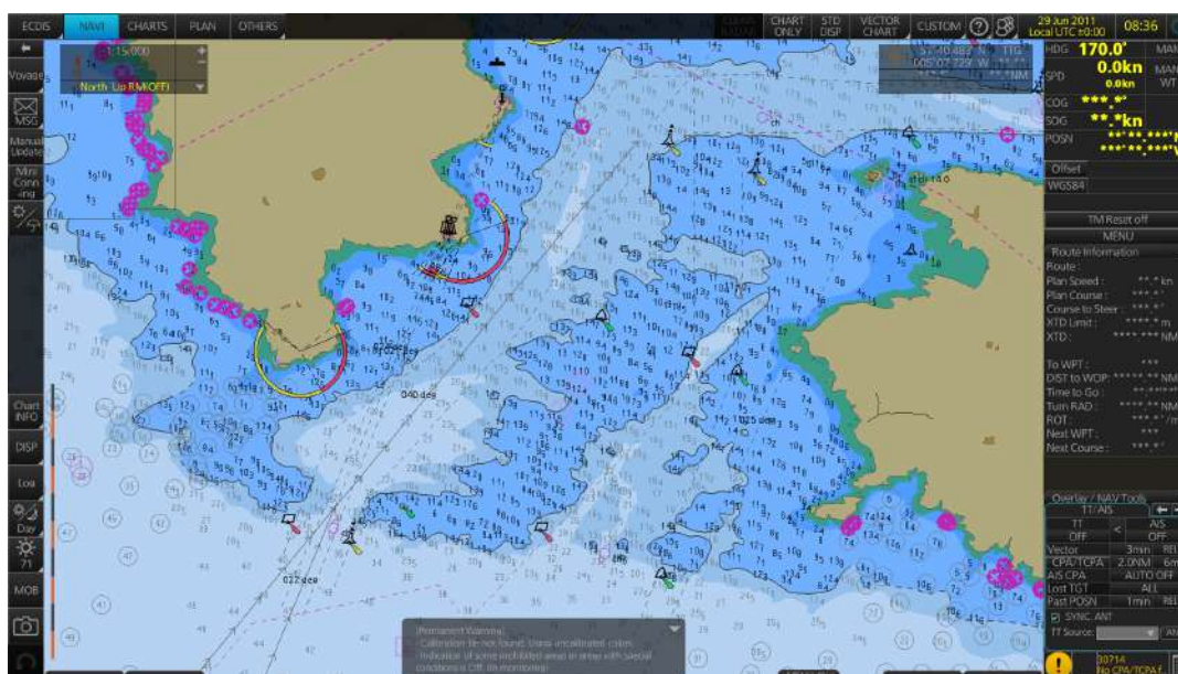
Figure 4.6: Example of ENC where the required 15m safety contour is available, using four-shade contours
