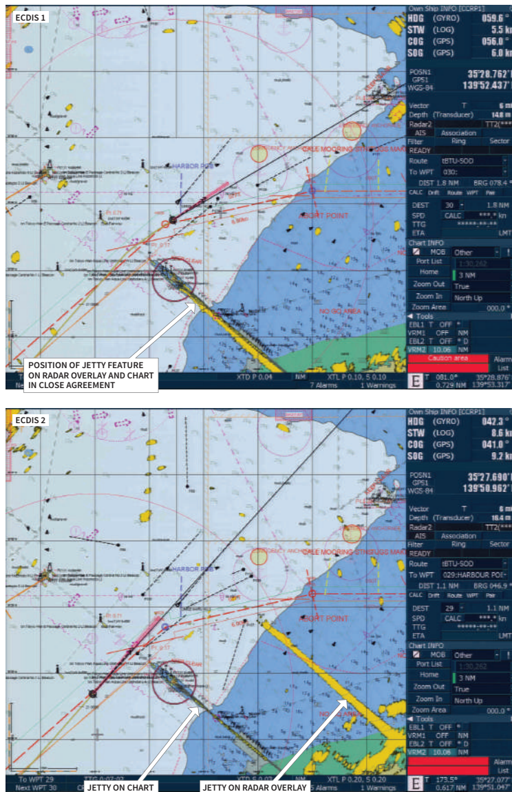
Figure 3: ECDIS screenshots illustrating radar overlay discrepancy
