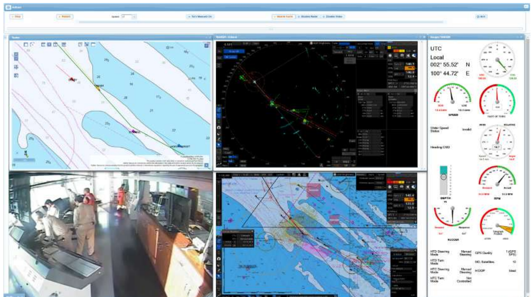
Figure 7: Replay of merged VDR and CCTV data
