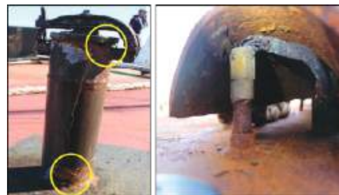
Figure 77. Postaccident photos of corroded no. 1 starboard cargo tank ullage tube (left) and wasted armored protected electrical cable with exposed wiring (right). SOURCE: COAST GUARD
