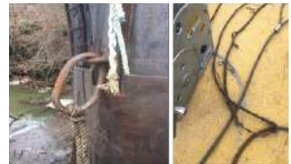
Figure 52. At left, a deformed anchor ring on third piling back from the forward piling at Jacks Run. At right, parted and frayed mooring wires from the lead shore-side barge during the accident.
