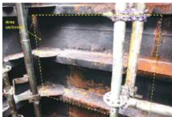
Figure 75. Cracks in bulkhead separating the forepeak from the port no. 1 cargo tank. The dashed section was removed and sent to the NTSB Materials Laboratory for analysis. SOURCE: COAST GUARD
