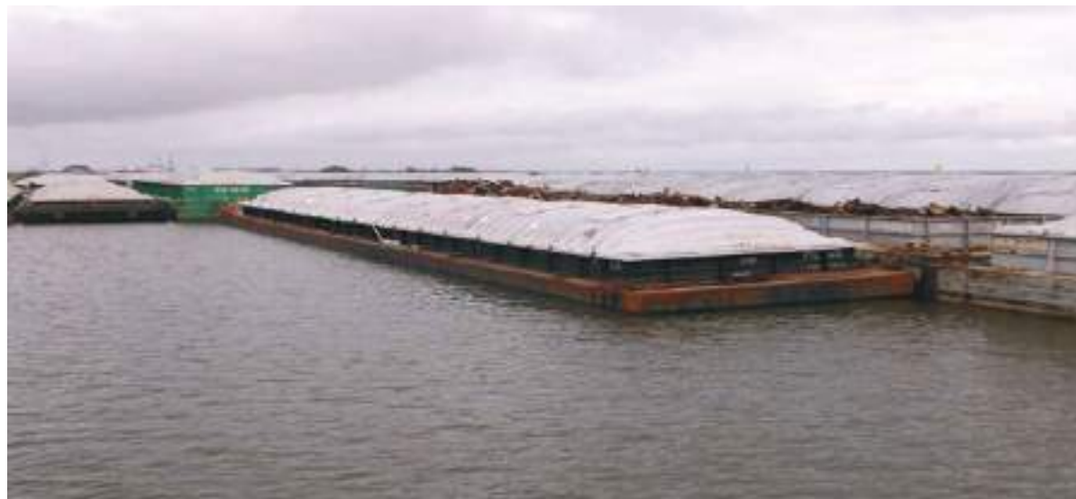
Figure 134. Barge PTC 625 (similar to PTC 598 ) with its fiberglass cargo covers closed.
