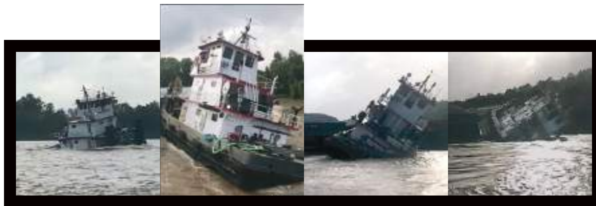
Figure 8. Sequence of events as the Miss Roslyn headed toward moored barges with a heavy list to starboard and eventually capsized. Left to right: (1) About 1650, the Miss Roslyn began crossing the Mississippi River with a noticeable list to starboard. As the vessel crossed the river, water increased on deck, and the vessel sank lower into the water. (2) The deckhands evacuate the Miss Roslyn . (3) About 1658, the vessel's list increases rapidly to starboard. (4) About 1659, the vessel lists further to about 90 degrees. SOURCE: CLAY HEBERT, ITV KRISTY DUTSCH
