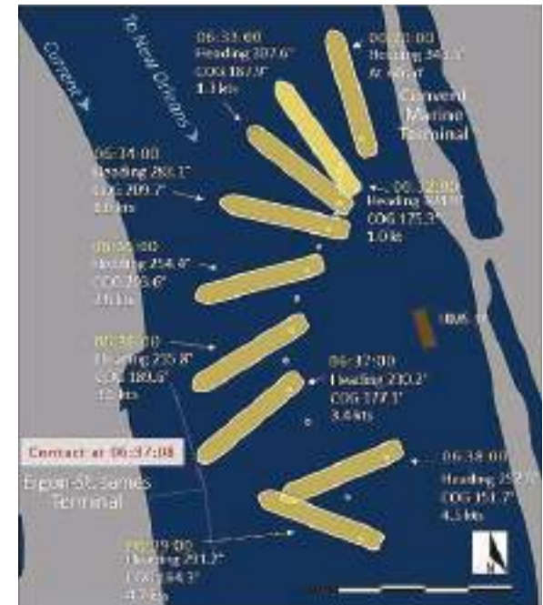
Figure 67. Trackline of the Shandong Fu En from 0620 to 0639, showing the vessel's heading and COG.
