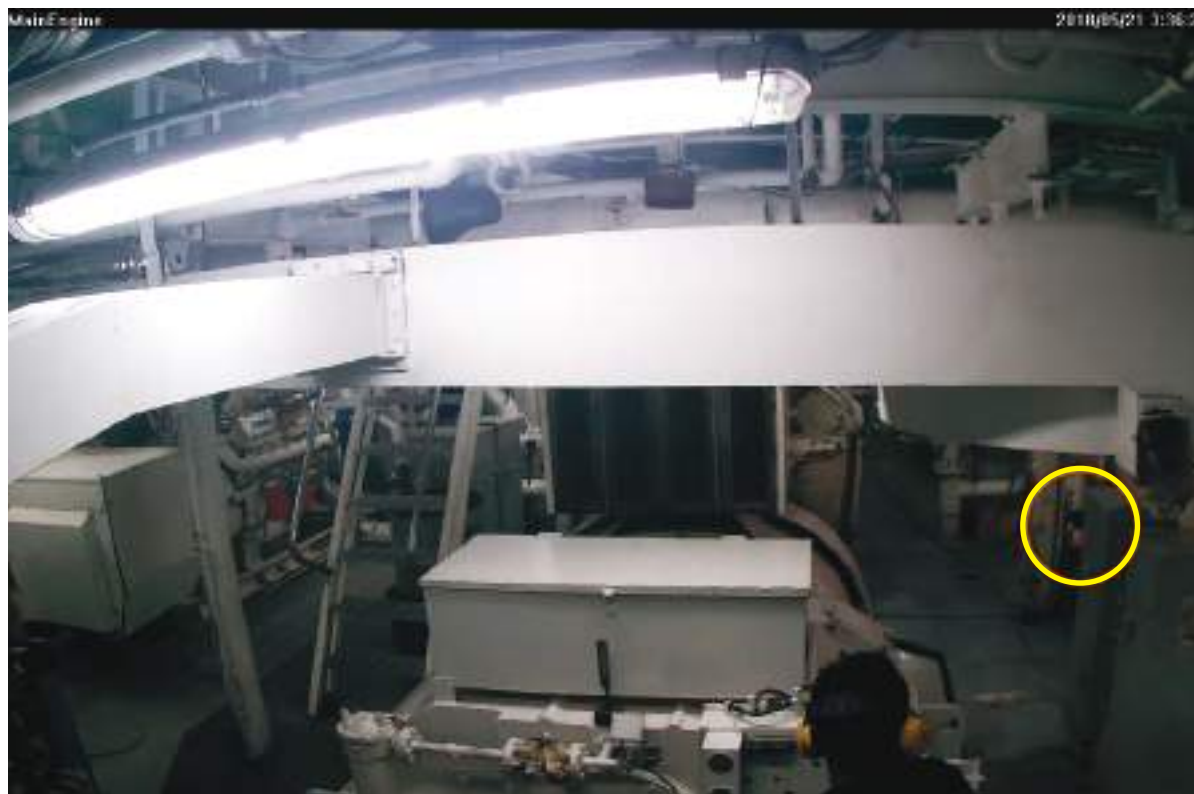
Figure 79. Screenshot from the closed-circuit television camera in the lower engine room, looking forward. The initial fire began in the area overlaid by a yellow circle (starboard side). SOURCE: COAST GUARD
