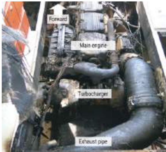
Figure 91. Damage to the engine as seen from above. Right: Damaged exhaust tubing after removal from engine room.
