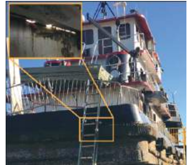
Figure 10. The orange outline approximate location of a large hole along the seam between the Miss Roslyn 's starboard steering void and aft main deck; the hole is shown in the inset image.
