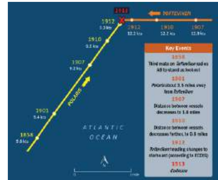
Figure 33. Tracklines of Polaris and Tofteviken leading up to collision, based on AIS data.
