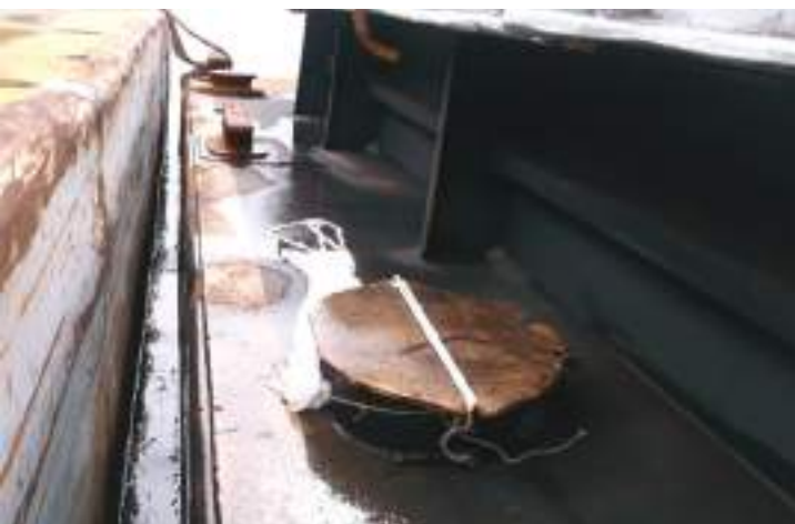
Figure 135. Postaccident views of a manhole cover on the PTC 625 is in poor condition, with missing dogs, and strapped down with line.
