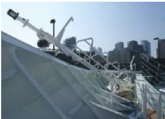
Figure 55. Carnival Horizon's damaged forward mast and support structure.
