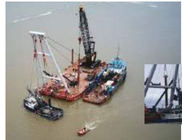
Figure 18. Pacific Knight while it was salvaged, with its crane positions visible in the inset.
