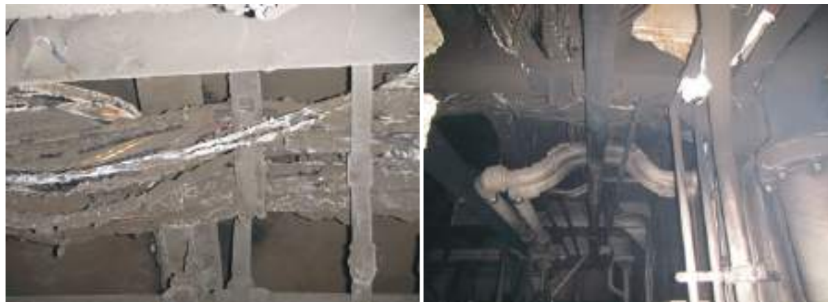
Figure 80. Left: Electrical cabling above generator no. 2. Right: Smoke and heat damage in the overhead of the starboard forward corner of the lower engine room. SOURCE: COAST GUARD
