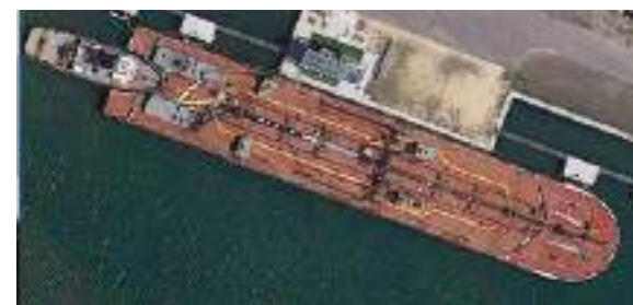
Figure 76. Overhead view of an ATB configuration. SOURCE: BOUCHARD TRANSPORTATION CO., INC.
