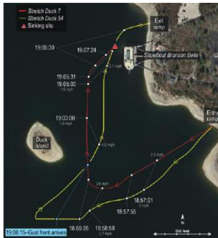
Figure 141. Vessel voyages on Table Rock Lake the evening of the accident. Red line represents the calculated trackline of the Stretch Duck 7 , and yellow line represents the actual trackline of the Stretch Duck 54 based on GPS data. 1
