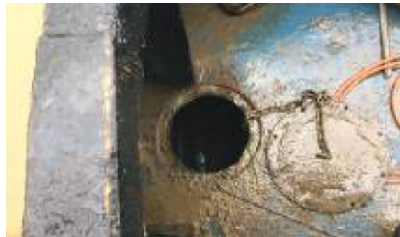
Figure 130. Starboard deck access to aft stern void found open during salvage, with broken and missing access cover screws.
