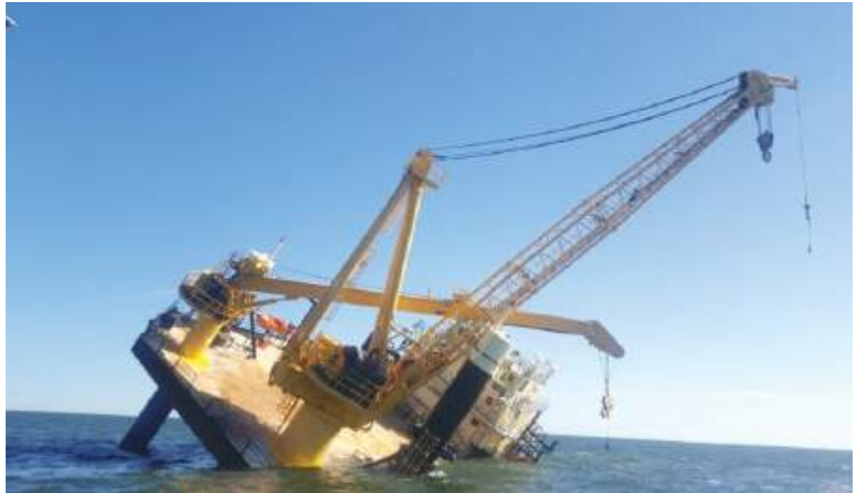
Figure 165. Ram XVIII after the vessel was abandoned, showing a significant angle of inclination to port.
