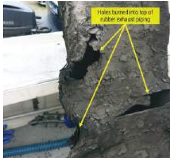
Figure 91. Damage to the engine as seen from above. Right: Damaged exhaust tubing after removal from engine room.
