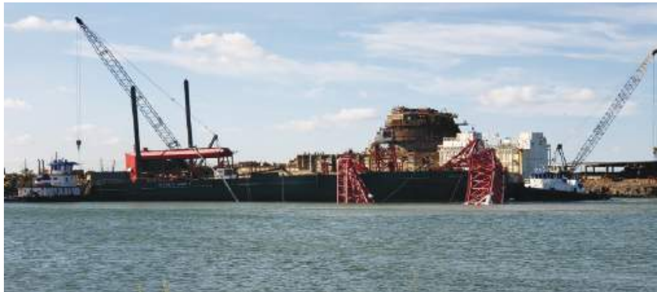
Figure 153. Collapsed crane boom on Atlantic Giant II . In background are TOPS DB1 and BOABARGE 29 .
