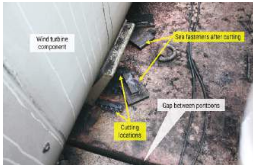
Figure 83. Left: Steel sea fasteners cut from deck in the portside no. 3 hold aboard Chipolbrok Moon , identified with yellow arrows. The gap between pontoons is also identified. SOURCE: HARRIS COUNTY FIRE MARSHAL
