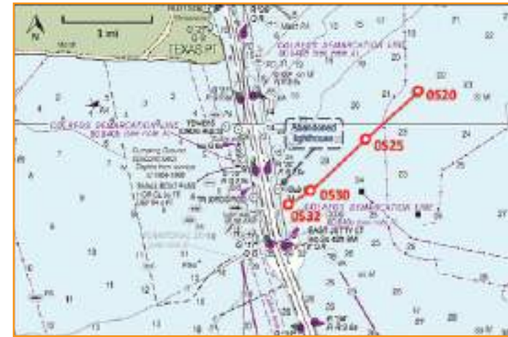
Figure 149. Trackline of the Capt. M&M before grounding on the jetty. SOURCE: NOAA CHART 11332
