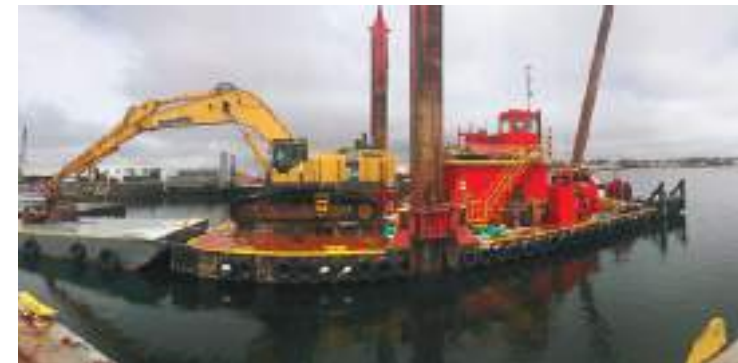
Figure 6. Dredge200 with excavator boom extended.
