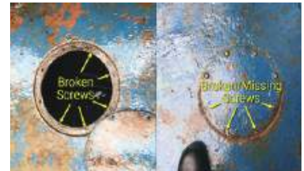
Figure 132. Starboard deck access to forward stern void found open during salvage. At right, port deck access to aft stern void, with broken and missing access cover screws.
