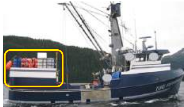
Figure 17. Left: the Pacific Knight while moored alongside a dock on June 10, 2018, with the two added cranes. Below: undated photo of the Pacific Knight (then named the Lone Fisherman ) with the aft deckhouse that was removed (highlighted in yellow). SOURCE: LONE FISHERMAN, LLC
