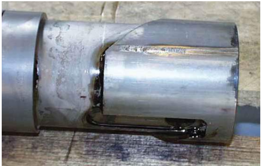
^ Fuel pump plunger scoring
