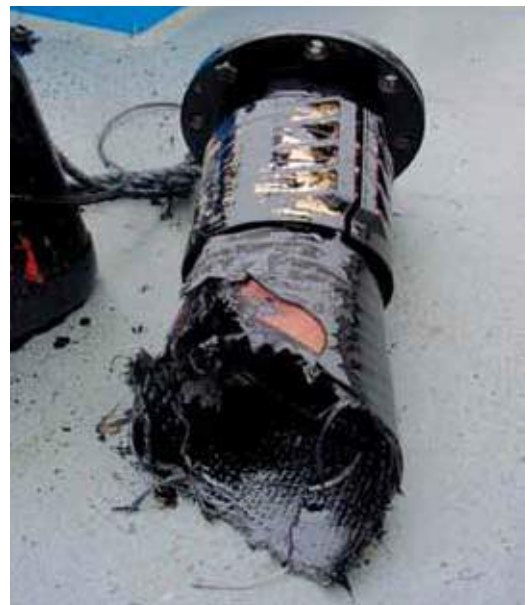
^ Failed bunker hose
