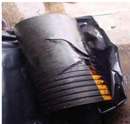
^ Cropped section of damaged bunker hose
