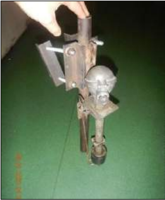
Figure 3: Bilge alarm sensor (representative photograph)
