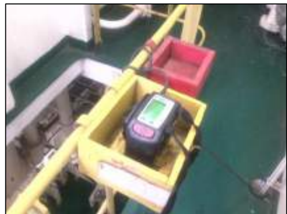
Figure 13: Portable gas detector replacing the personal multi gas detector
