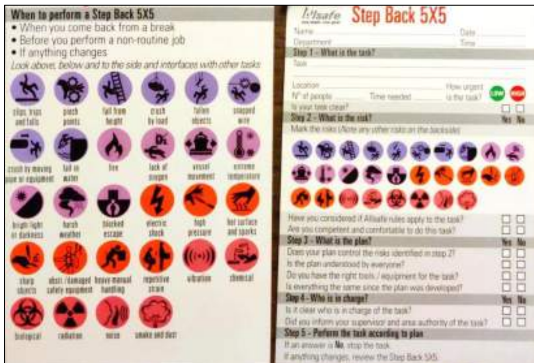
Figure 14: Step-Back 5x5 pocket cards used on board for in-situ risk assessment
