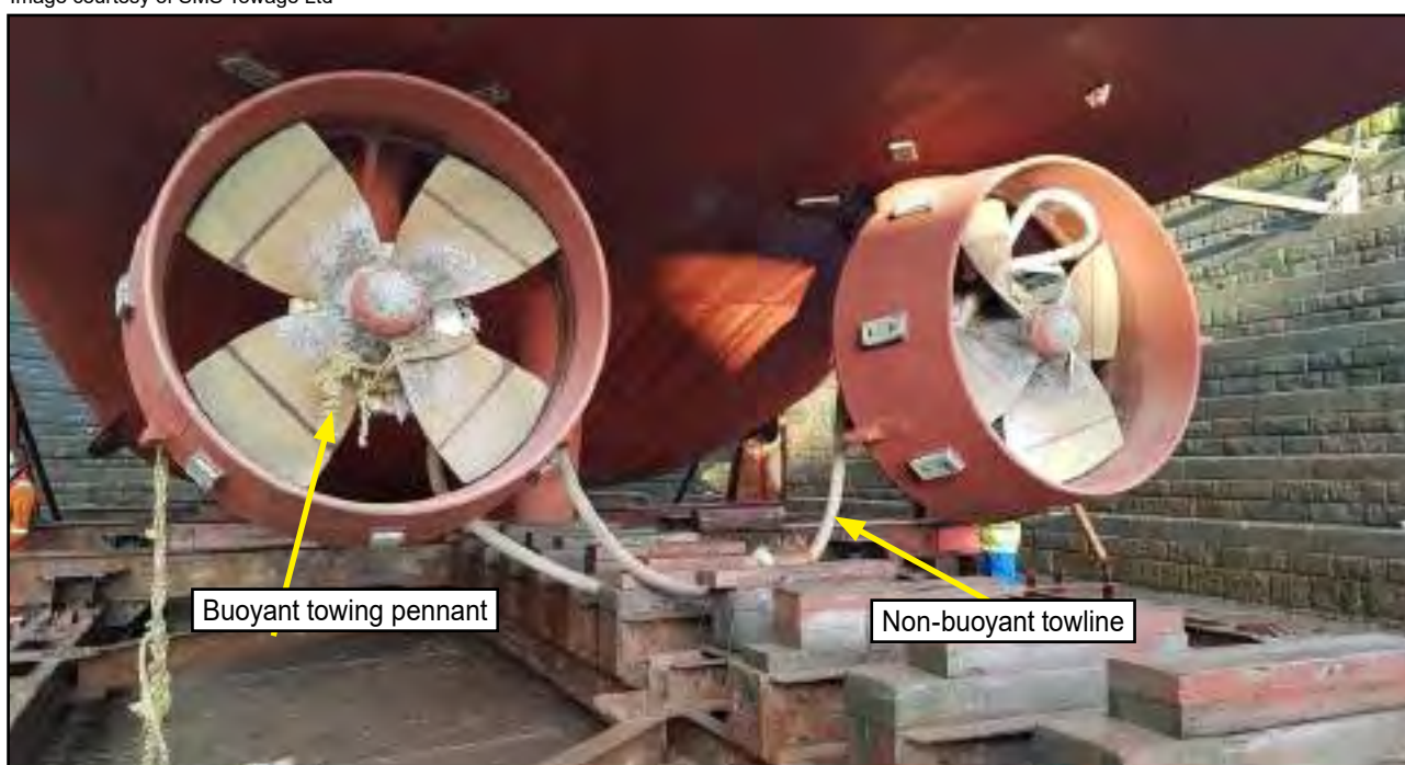
Figure 7: Yeoman's propellers fouled by Svitzer Josephine's towline
