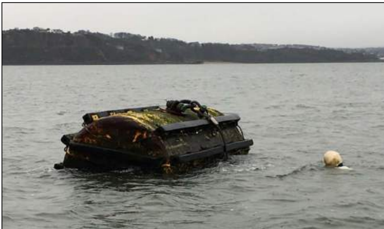
Figure 1: Unlit mooring buoy, with significant marine growth
