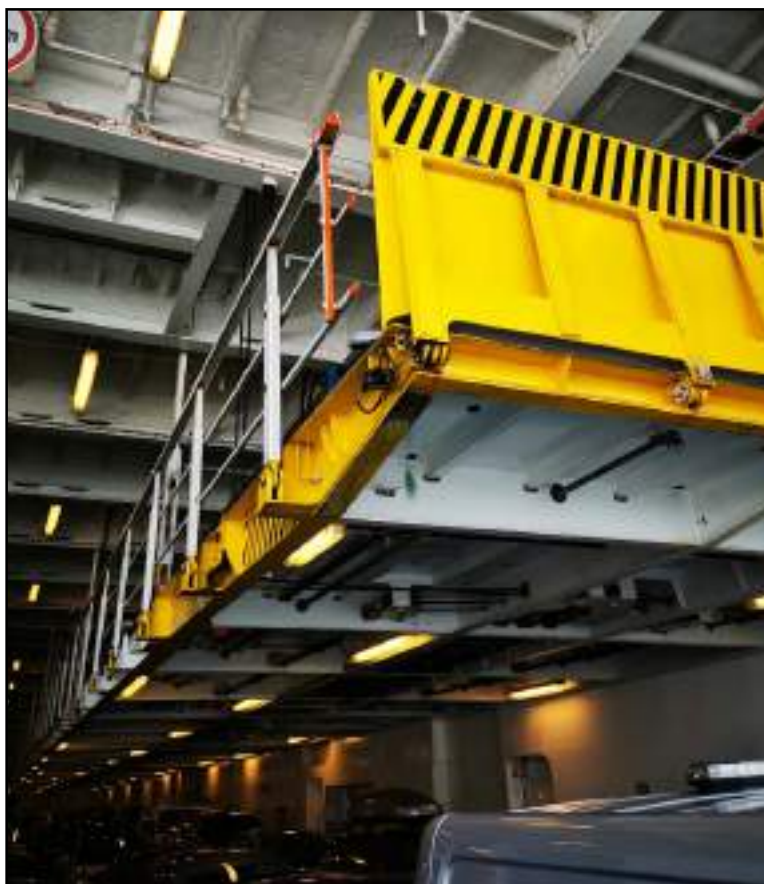
Figure 1: The loaded mezzanine decks in the raised position with the vehicle ramps in the vertical (safe) configuration
