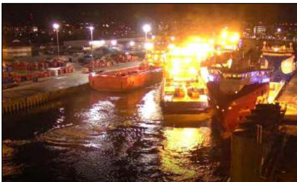
Figure 3: Loss of control and sheer to port, with contact made with berthed vessels
