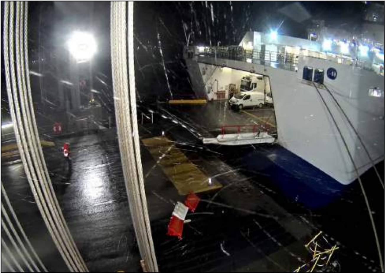
Figure 3: View of stern of ship being blown across linkspan
