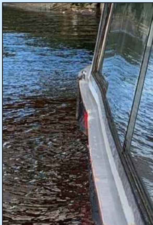
Figure: Damage to the passenger vessel's port side after the contact with the bridge
