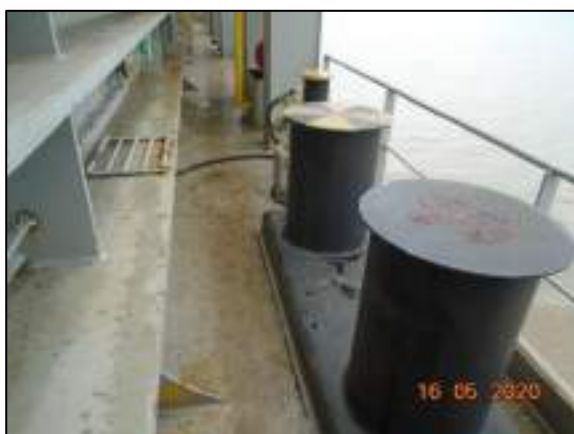
Figure 1: Mooring bitts where the tug's line was made fast for departure
