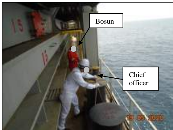
Figure 2: A photo simulation of the bosun holding on to the pick-up gear and the chief officer clearing the eye of the tug's line from the mooring bitts
