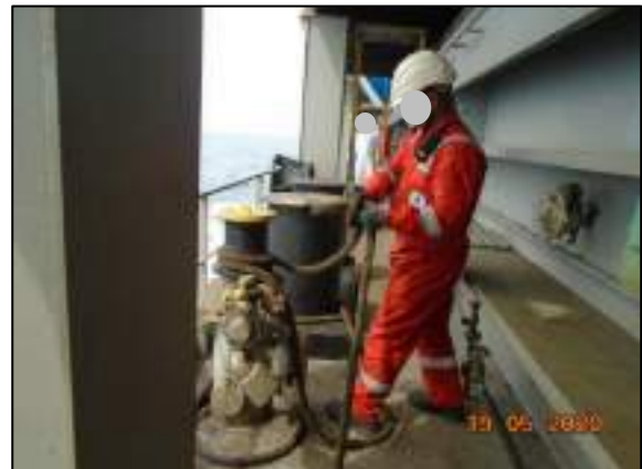
Figure 4: A photo simulation of the bosun attempting to disconnect the messenger line and the pick-up gear
