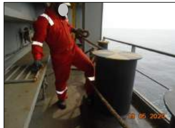
Figure 5: A photo simulation of the bosun's left leg getting caught in between the pick-up gear and the mooring bitts
