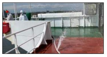
able to deliver the required two jets of water due to malfunctioning impellers. The ship had to run both pumps simultaneously to supply enough pressure. Finally, despite only two issues related to inoperable smoke detectors, there were still a few deficiencies related to smoke detectors being found covered with plastic bags.
