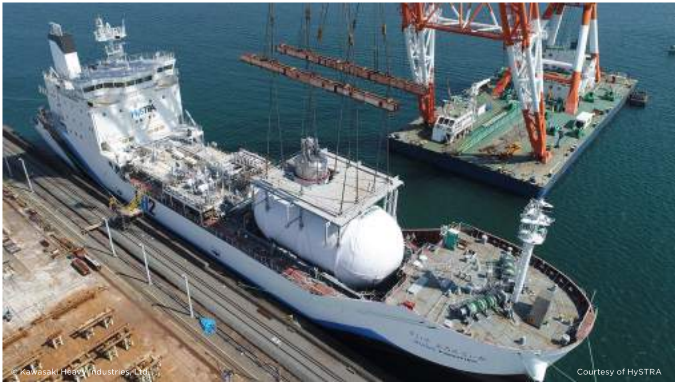
Figure 15: The Suiso Frontier is the First Liquid Hydrogen Carrier, Launched in 2021 and Intended for Use in the HESC
