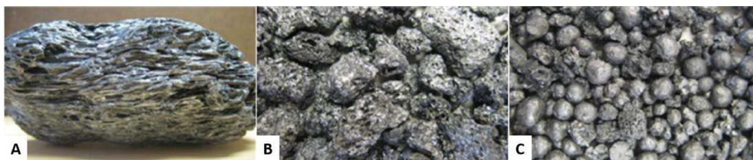
**Figure 1.** Some of the petcoke types. **A.** Needle petcoke; **B.** Sponge petcoke; **C.** Shot petcoke. Source (Edwards, 2015)<sup>2</sup>.
