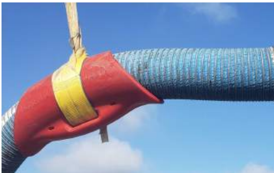
Figure 5.3: Example of a proprietary Hosebun device
