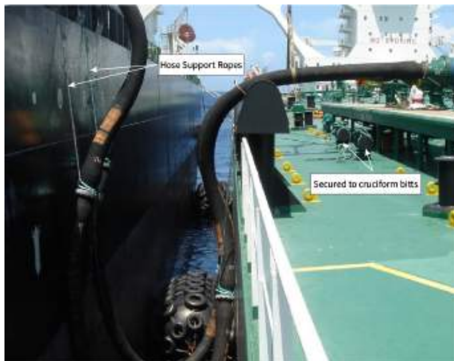
Figure 5.2: Hose support ropes passed through fairleads and secured to cruciform bitts
