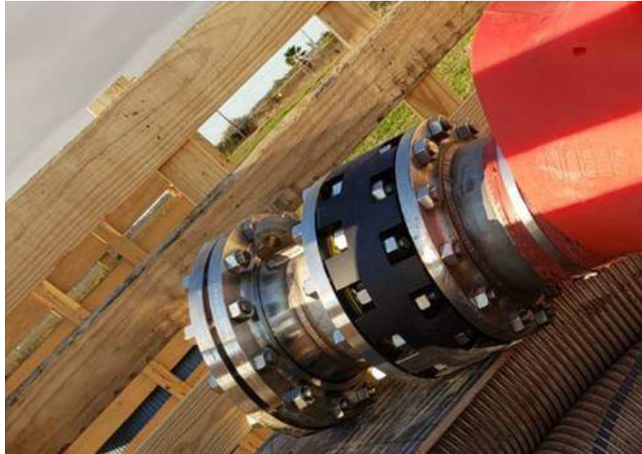
Figure 5.6: Example of a Type 2 Insulator – insulating block
