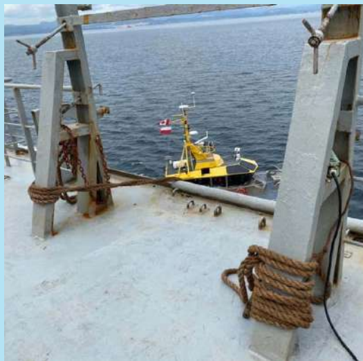
Pilot ladders should never be affixed to non-designated securing points such as seen here.
