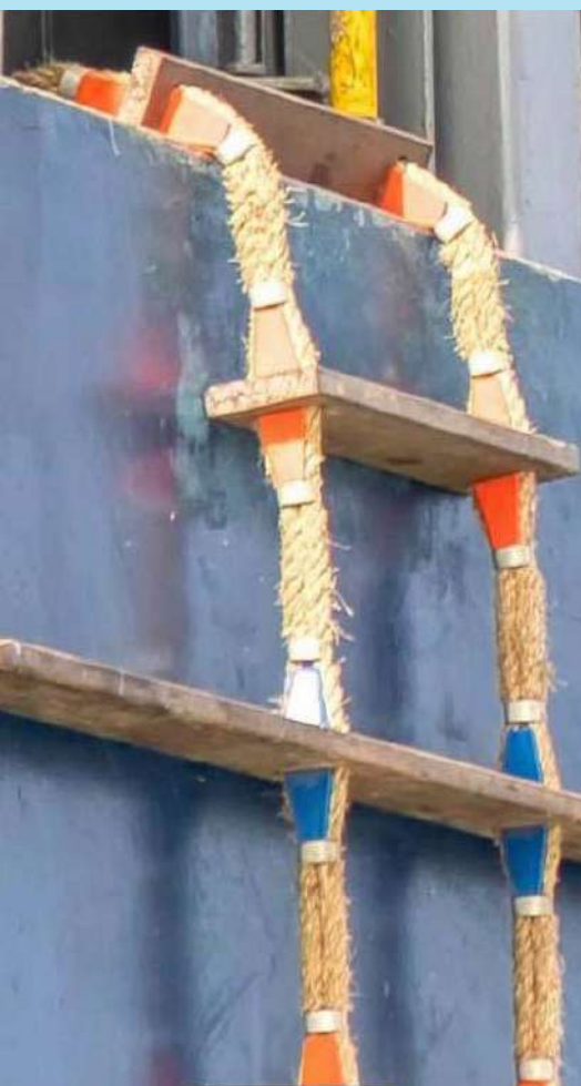
Pilot ladder over the side across a sharp edge.
