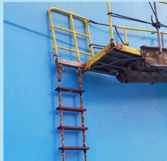
Pilot ladder is to be secured to the ship, not the accommodation ladder.
