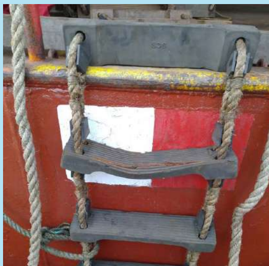
These pilot steps have seen many feet cross them and should be replaced.
