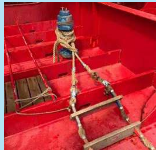
Pilot ladders should never be affixed to non-designated securing points such as seen here.
