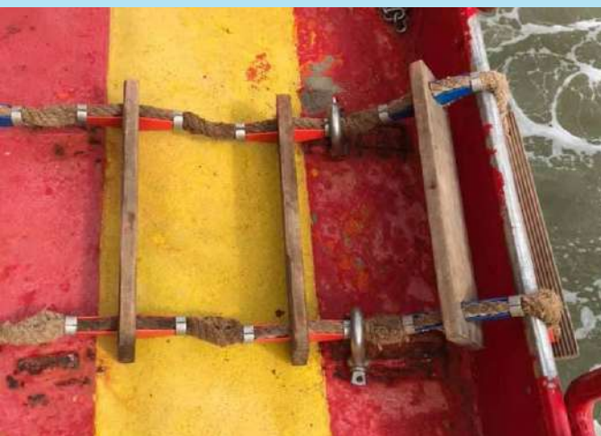
Steel shackles used to secure pilot ladder side ropes should also be avoided as they are not reliable to handle the weight and will damage the chocks.
