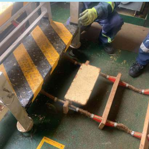
Affixing a deck tongue over a pilot ladder should be avoided as they are not designed to carry the load of the ladder.
