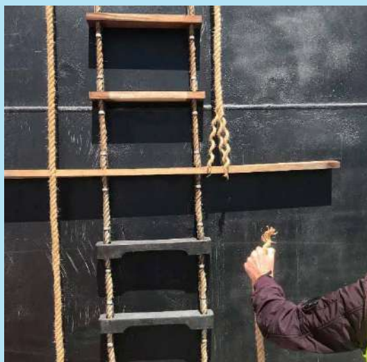
Frayed and broken man-rope.
