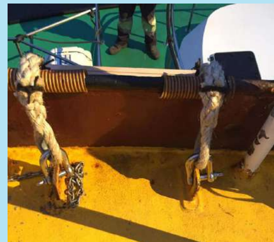
Well designed pilot station with a section of cut steel pipe affixed to ensure pilot ladder goes over a rounded edge.
