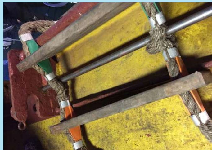
The use of steel bars to secure pilot ladders should also be avoided as they are strung through side ropes the can damage the ropes that are not designed to carry such loads at such points.
