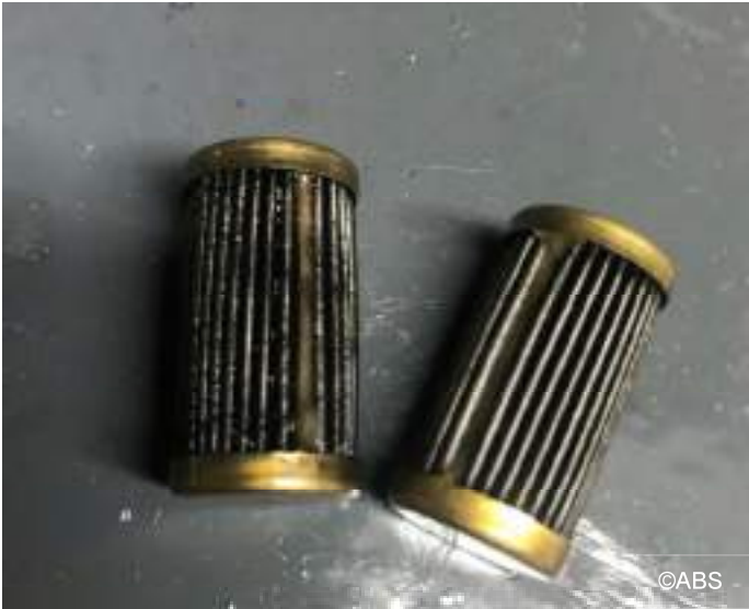
Main engine shut down due to clogged fuel injector screens
