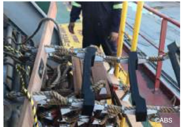
New pilot ladder provided
