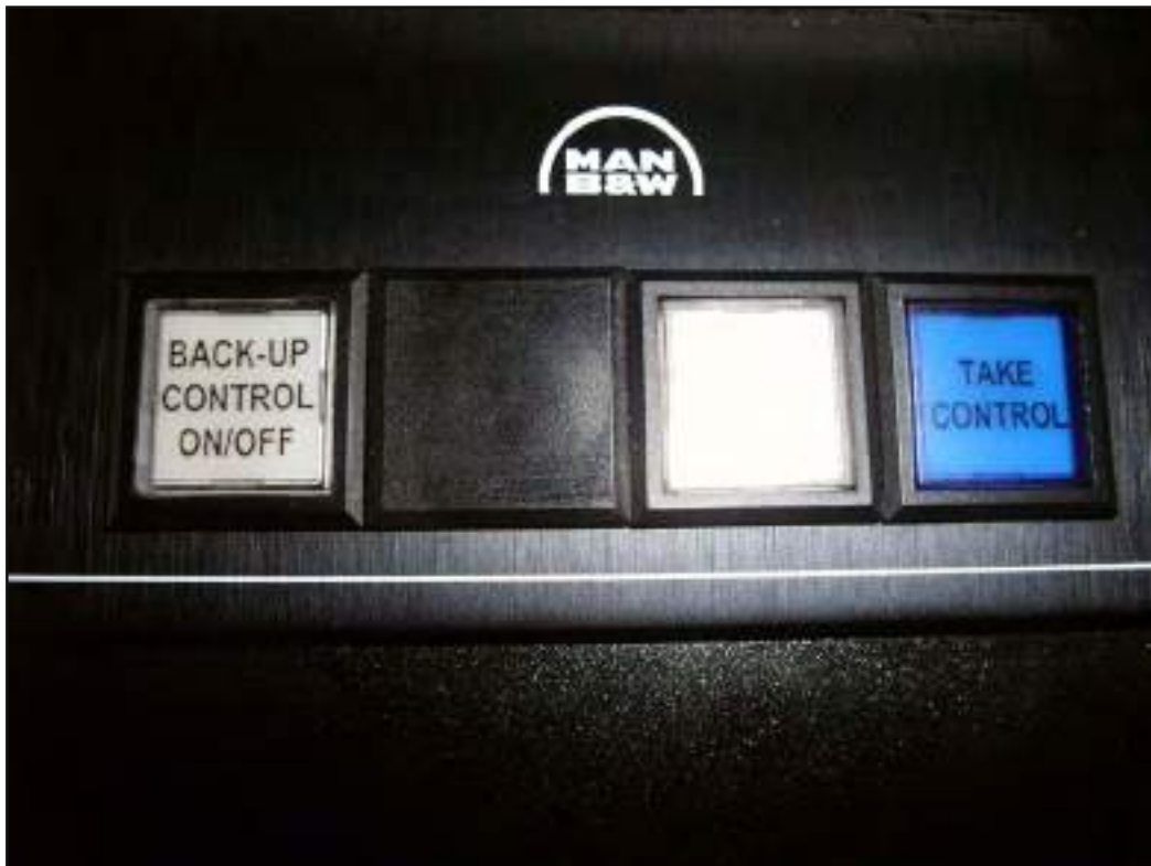
Figure 7: Backup control to bypass the AT2000 PCS
