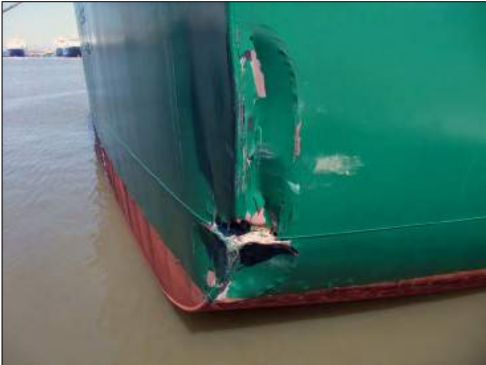
Figure 2: Damage to Saffier
