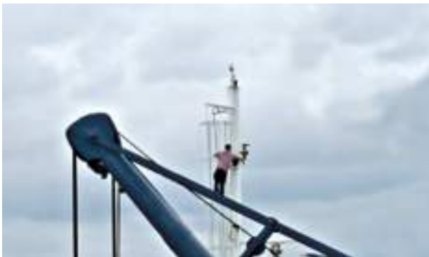
Working aloft with no safety harness or PPE
