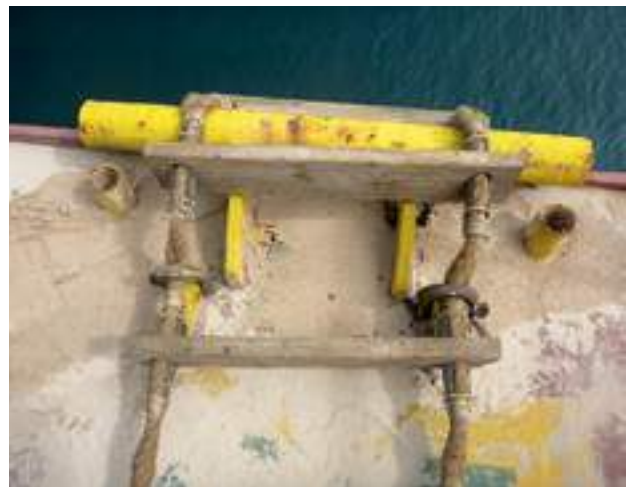
Pilot ladder incorrectly secured to the deck using D-shackles to choke the side ropes.
