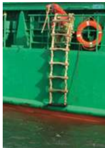
Notorious offender with bulwark setup. It's not even a pilot ladder (at least 6 non compliances).
