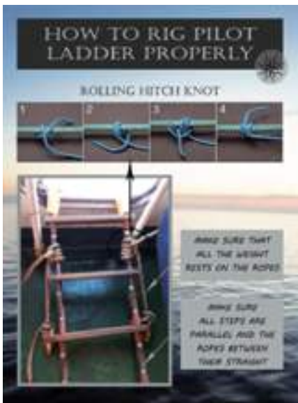
How to secure the pilot ladder correctly at deck level.
