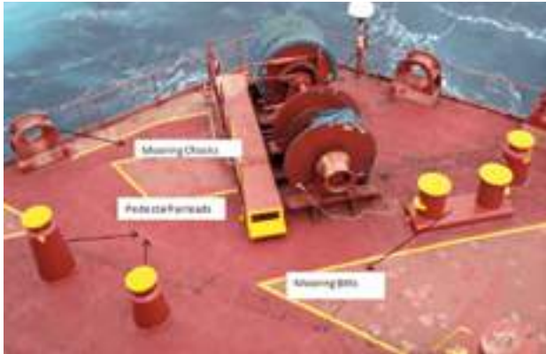
Example of a typical modern mooring arrangement (Not the vessel in the report)
