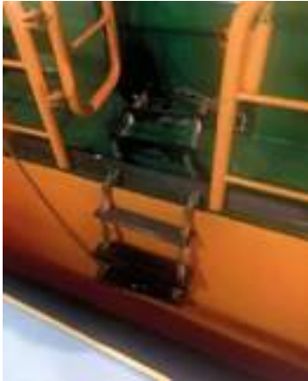
Another spreader used as a securing method.
