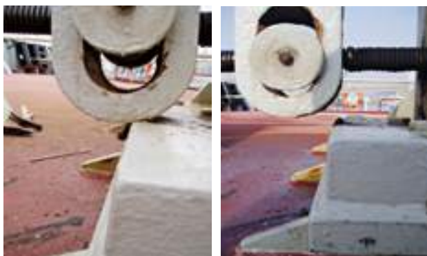
Incorrect Brake Adjustment Correct Brake Adjustment
