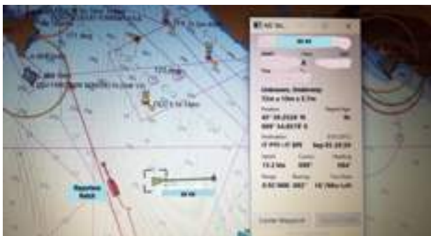
Screen shot of AIS display after the round turn to starboard
