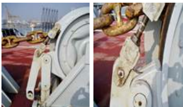
Brake 'Fully On' Bottle Screw Adjustment
