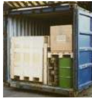
Figure 7.28 Mixed stow, use of pallets
