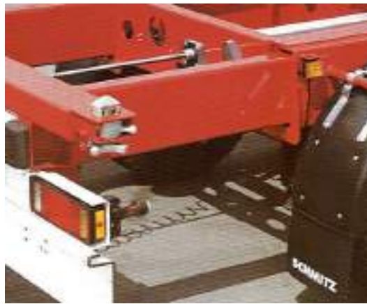
Figure 2.1 Twistlock on a road vehicle
