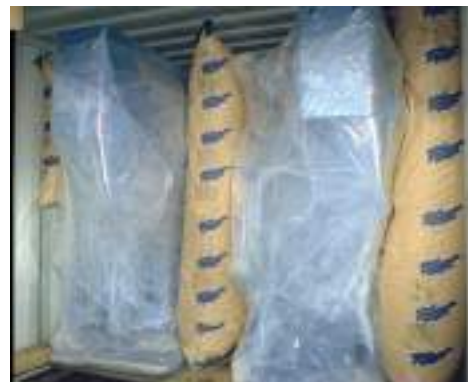
Figure 7.10 Irregular shaped packages blocked with dunnage bags
