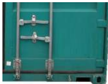
Figure 5.27 Handles between bars
