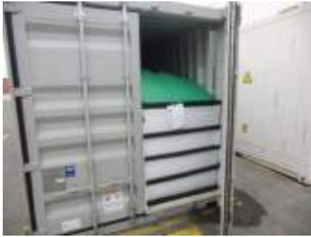
Figure 7.51 Container fitted with flexitank
