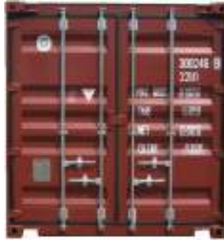
Figure 4.7 Rear of freight container
