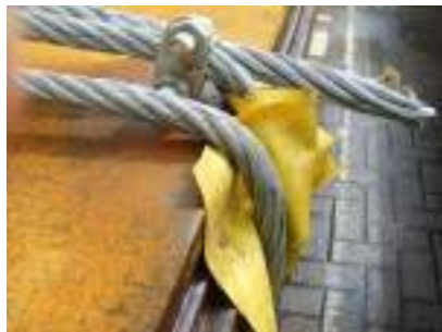
Figure 7.11 Poor edge protection
