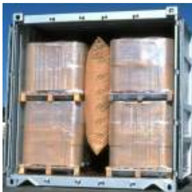
Figure 7.9 Gap filled with a central dunnage bag
