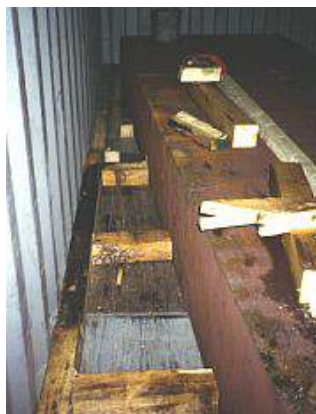
Figure 7.45 Transverse blocking of steel slab
