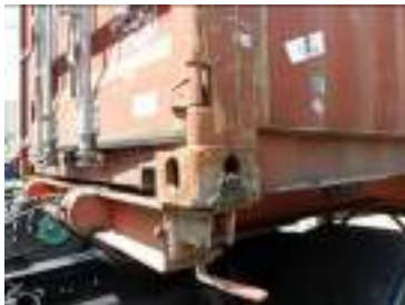
Figure 6.2 Mud in corner fitting
