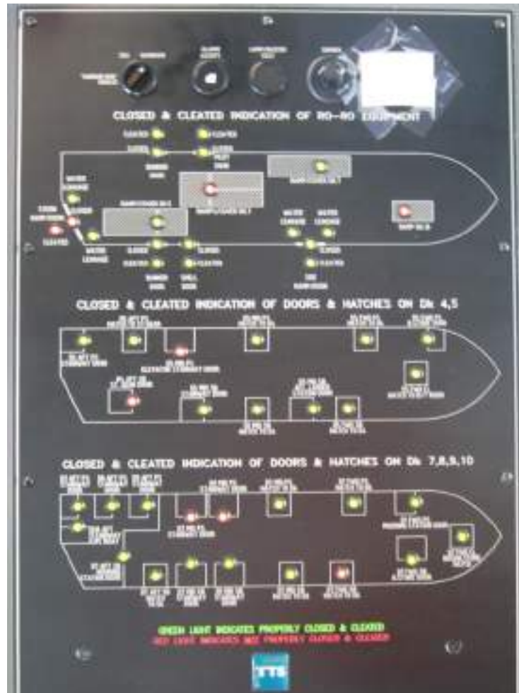
Figure 10. Watertight door indicator panel located on the bridge of the Silver Ray , a vessel of the same class as the Golden Ray .
