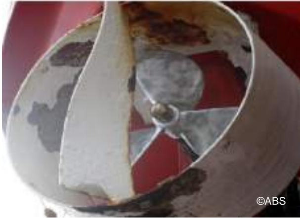
Lifeboat rudder corroded - before
