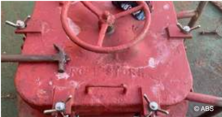
Watertight booby hatch with new dog bolts
