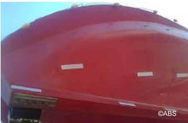
Lifeboat reflective tape replaced
