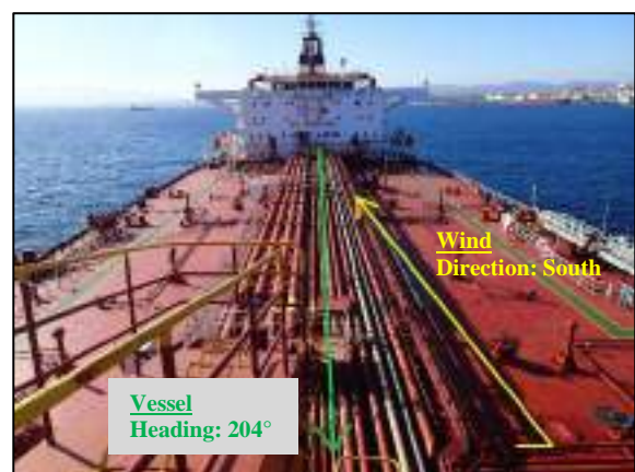
Figure 6: Wind direction relative to the vessel's heading
