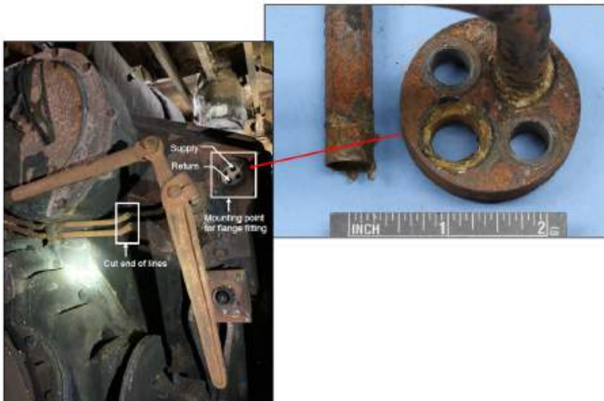
Figure 9. Starboard main engine after the fire with section of fuel oil supply and return lines removed ( left ). Laboratory image of flange and de-brazed and separated fuel oil return line ( right ).
