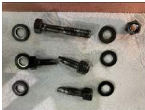
Figure 8. Damaged lower basket bolts, washers, and nuts from no. 3 main engine's nos. 6 and 14 connecting rod and piston pair. (Source: WSF)
