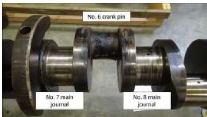
Figure 6. Damaged crankshaft from no. 3 main engine. (Source: Dynamark Engineering)
