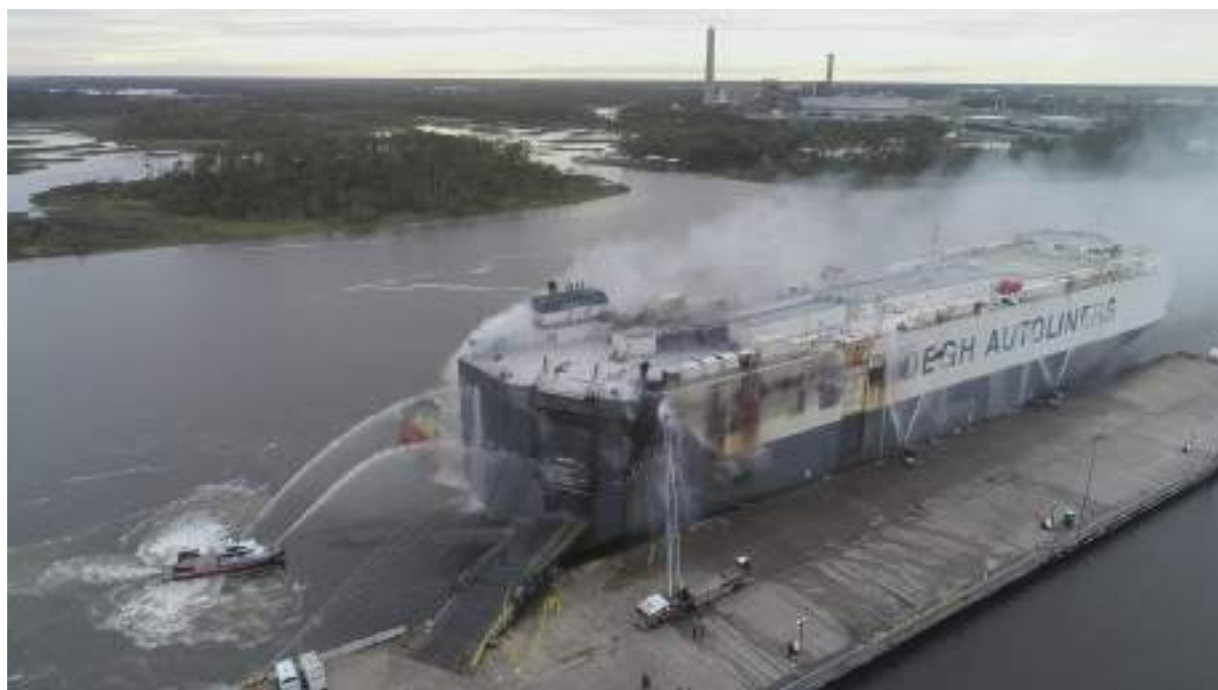
Figure 6. Firefighters conducting exterior boundary-cooling on June 5, 2021, the day after the fire was discovered. (Source: JFRD)
