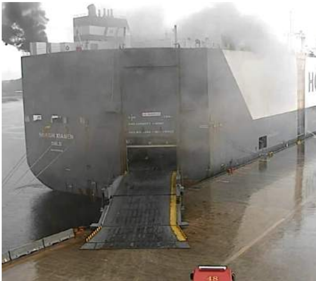
Figure 16. Engine 48 arriving on scene about 1603. Starboard vents 10/11E and 7/8E and port vents 10/11E and 9E exhibit smoke flow. (Source: Jacksonville Port Authority)
