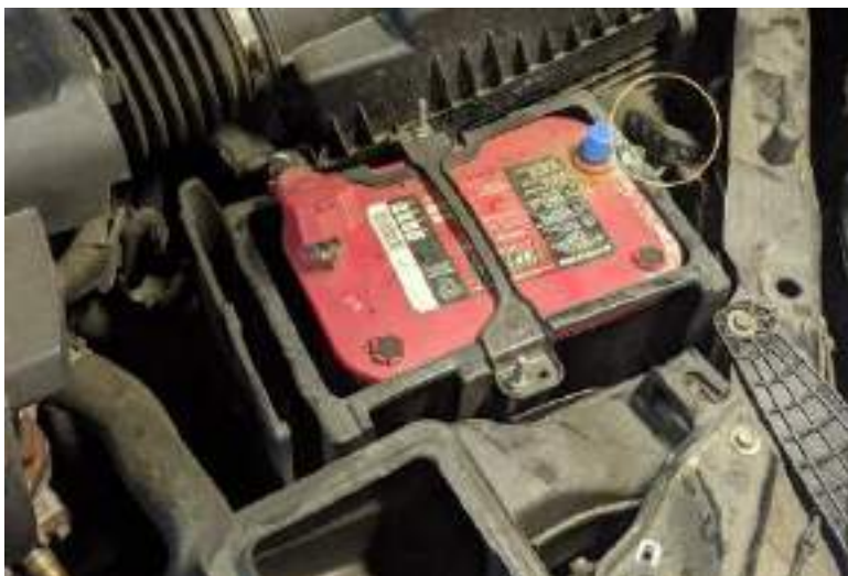
Figure 12. Excerpt from Grimaldi battery disconnect procedure showing a vehicle battery secured with a blue plastic negative terminal cap and disconnected cable ( circled ) tucked inside. (Source: Grimaldi)
