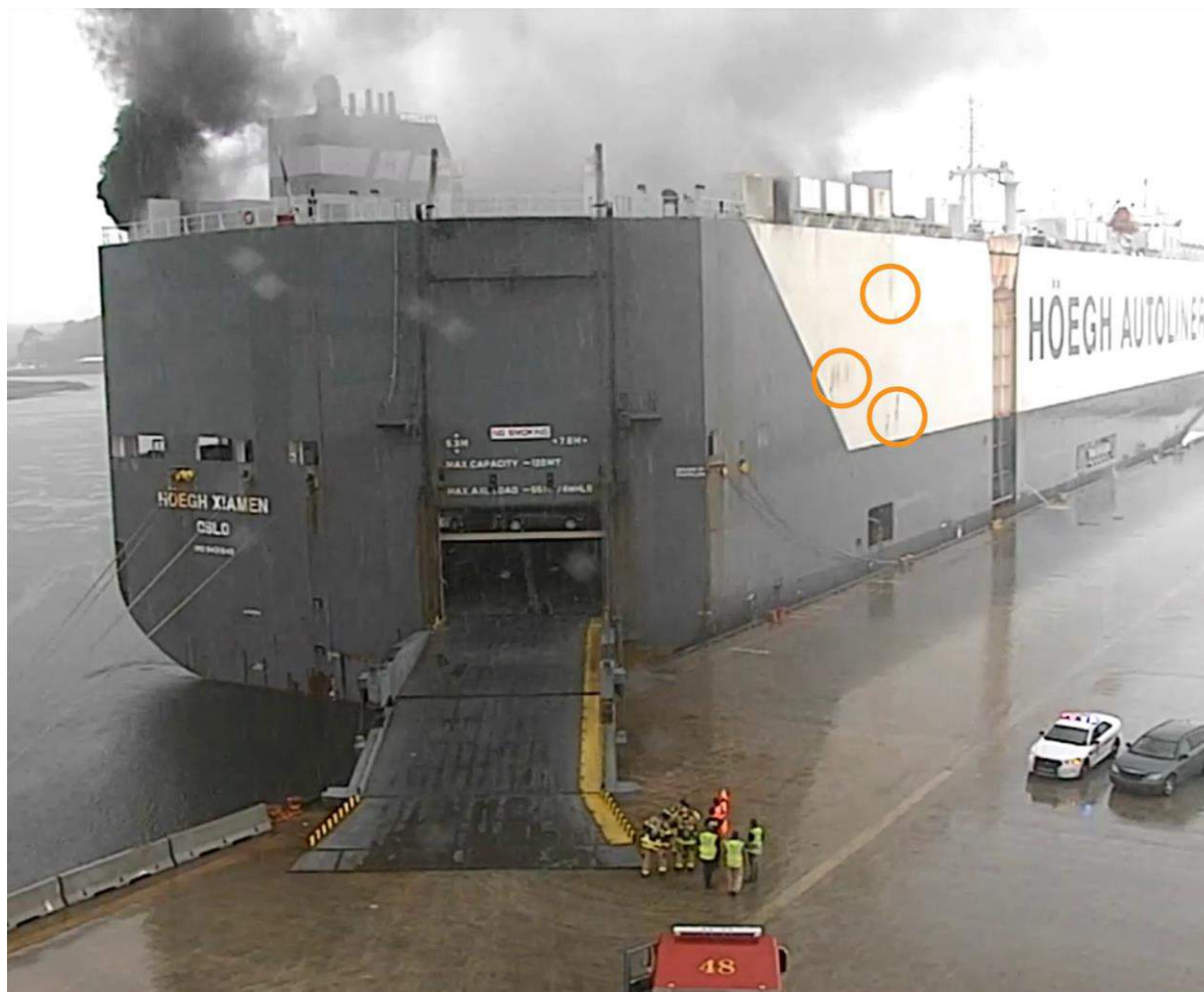
Figure 17. About 1608, 5 minutes after Engine 48's arrival, the white paint on the starboard side of the vessel exhibits thermal discoloration (circled in orange). Starboard vents 10/11E and 7/8E and port vents 10/11E and 9E exhibit smoke flow. (Source: Jacksonville Port Authority)
